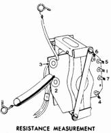
RESISTANCE MEASUREMENT Between terminal 1 & 2-138 Ohms Between terminal 2 & 3-420 Ohms Between terminal 7 & 7-2.2 Ohms Between terminal 7 & 5-7.3 Ohms Between terminal 5 & 6-3.8 Ohms
