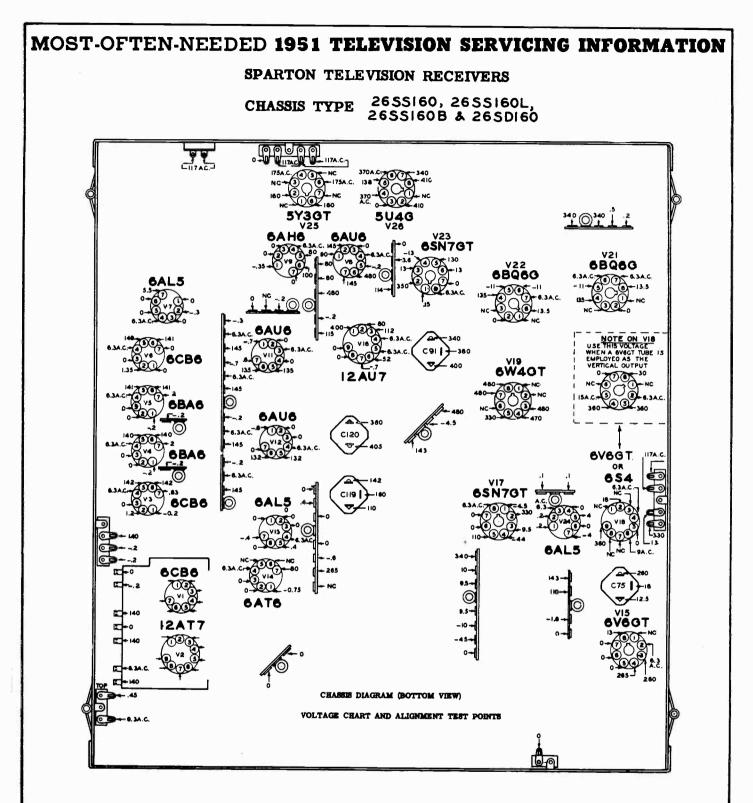
Unless otherwise indicated, the voltages shown in the above chassis diagram were measured in respect to chassis ground. The line voltage at 117 volts A.C. Set for no signal on Channel 2. Brightness and contrast set for maximum (clockwise). Volume and tone controls set at maximum counter-clockwise. Other controls set for proper operation. Measurements made with a vacuum tube voltmeter.
