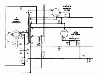
When replacing a #508679 transformer with a #508971 transformer, or vice versa, the following circuit changes must be made in addition to noting differences in terminal connections.
