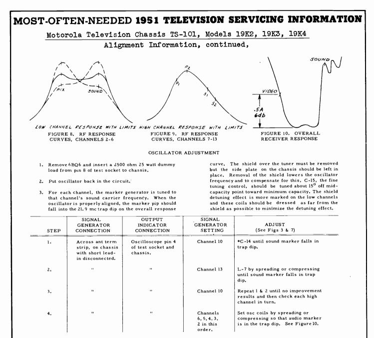
\* C-l4 is adjusted on channel 10 since this is mid-channel of channels 7-l3. All high channels must be checked to be sure that they fine tune within plus or minus 30 degrees of the setting of the fine tuning capacitor as explained above.
