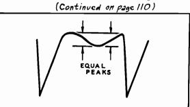
Figure 1. Horizontal Sweep—Horizontal **Stabilizing Core Properly Adjusted**
