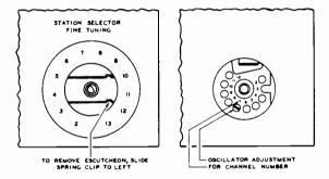
Figure 3-R-F Oscillator Adjustments
