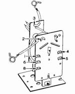
RESISTANCE MEASUREMENT Between terminal 1 & 2-- 40 Ohms Between terminal 2 & 3--400 Ohms Between terminal 5 & 8-- 11 Ohms Between terminal 6 & 8-- 5.5 Ohms 508679
