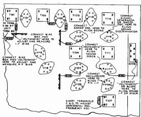
Figure 10-Test Connection Points
