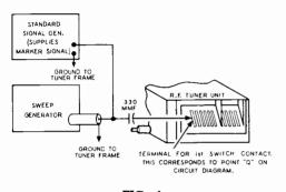
FIG. 4 Generator Connections for IF Channel Alianment Detailed information in table form on I.F. alignment is given on the next page. Some pointers on sound, R.F., and oscillator alignment can be gathered from this page.
