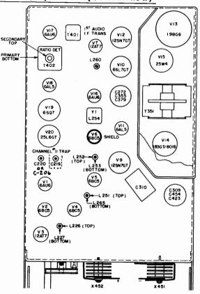
Fig. 22. Tube and Trimmer Location
