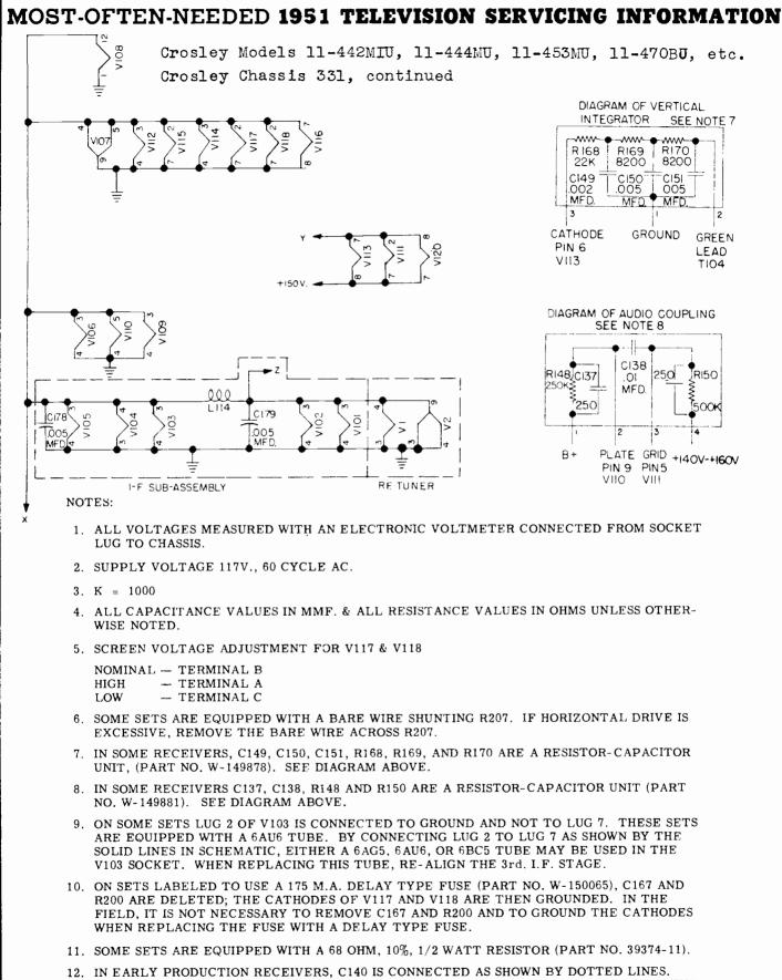
12. IN EARLY PRODUCTION RECEIVERS, C140 IS CONNECTED AS SHOWN BY DOTTED LINES. IN LATER PRODUCTION SETS, C140 IS CONNECTED AS SHOWN BY SOLID LINES TO PREVENT PARASITIC OSCILLATION IN THE AUDIO OUTPUT TUBE.
