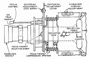
Figure 1-Yoke and Focus Magnet Adjustments
