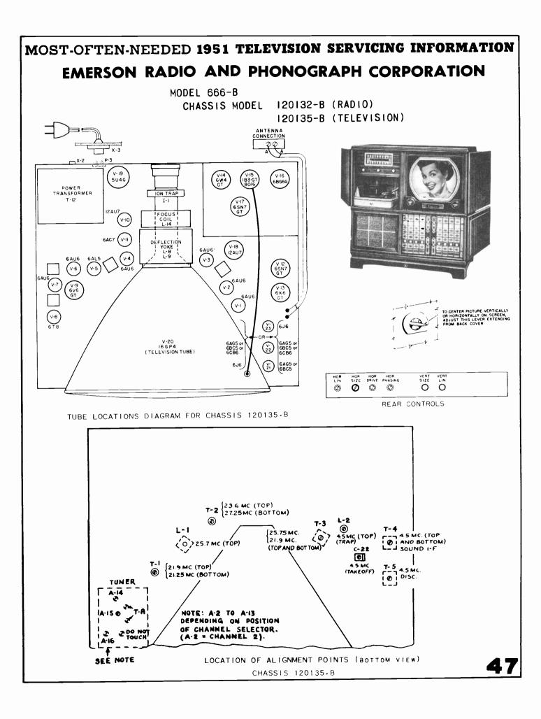
Emerson Radio, Television Chassis 120135-B, used in Model 666-B
