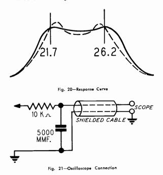
C. With same I-F sweep input, connect scope probe to second detector (junction of peaking coil (L-9) and 4700 ohm resistor (R-31) off Pin 7, 6AL5). Input should be adjusted to give 2 volt P to P output. Apply 3 V, bias (dc) to AGC line. (battery).
