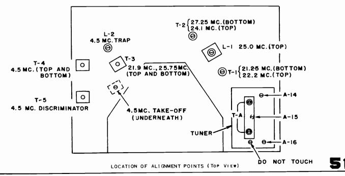
Emerson Radio, Chassis 120129-B Television Schematic Diagram
