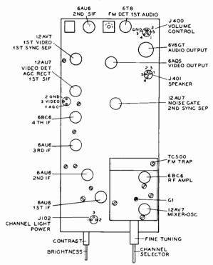
Figure 3. R-F, I-F Chassis, Top View
