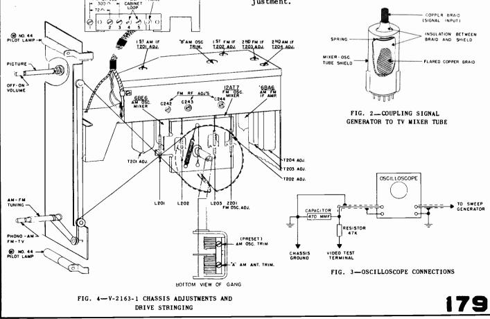
Westinghouse Electric Models H-633C17 and H-634C17 Alignment Procedure
