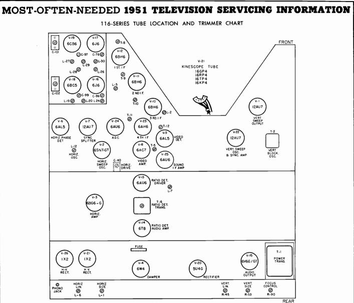
2. The output from the sweep generator is coupled into the plate of the Lo Band converter tube V-17, 6J6, by means of the special tube shield. This special shield is constructed by cutting tube shield SC No. 151036 in two,  $\frac{34}{2}$ " from the base. Separate the two pieces by  $\frac{1}{2}$  want secure by soldering 4-1 meg. ohm  $\frac{1}{2}$  watt carbon resistors to each part as shown below.
