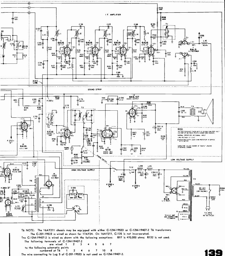
The wire connecting to Lug 5 of C-201.19533 is not used on C-12M-19407-2.
