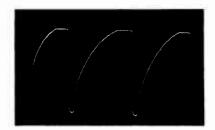
Fig. 20. Horizontal-Output Grid, Pin 5, 160 volts, 15,750 c.p.s.
