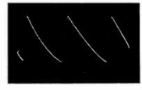
Fig. 16. Phase Comparer, Pin 6, 7 volts, 15,750 c.p.s.
