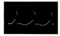
Fig. 19. Horizontal-Oscillator Grid, Pin 2, 40 volts, 15,750 c.p.s.
