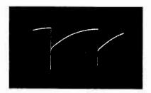
Fig. 14. Vertical-Output Grid, Pin 2, 72 volts, 60 c.p.s.
