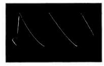
Fig. 16. Phase Comparer, Pin 2, 11 volts, 15,750 c.p.s.
