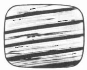
Figure 13. Picture Out of Horizontal Sync.
