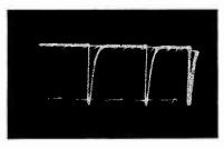
Fig. 12. Sync Separator Plate, Pin 5, 41 volts, 15,750 c.p.s.
