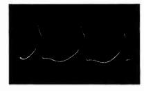
Fig. 19. Horizontal-Oscillator Grid, Pin 2, 65 volts, 15,750 c.p.s.
