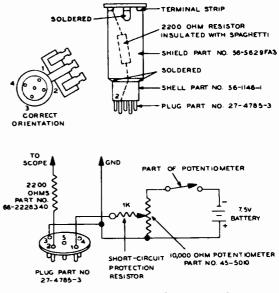
Figure 2. Video I-F Alignment Jig
