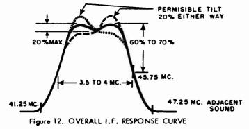
NOTE: It may be impossible to observe the 47.25 MC. marker with the average service equipment due to the high attenuation of trap L-1 (adjacent sound).
