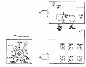
Figure 4. Television Tuner, Showing Locations of Adjustments
