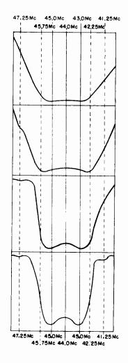
FIG. 6 – RESPONSE CURVES AT VARIOUS STAGES OF ALIGNMENT
