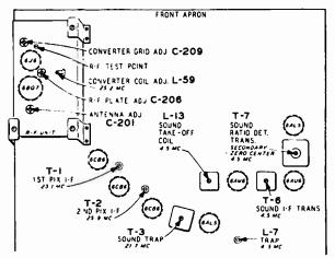
A. Unmodulated R-F signal into Converter Grid by means of tube shield insuloted from bose. VTVM with filter in lead of 22 K ohms and 5000 mmf connected to pic. det. load resistor, (R-100) 4700 ohms, in series with peaking coil (L-6) from Pin 7 of 6AL5. Input signol level should be such that output is less thon 2 volts DC. Apply -4.5V battery bias on AGC line.
