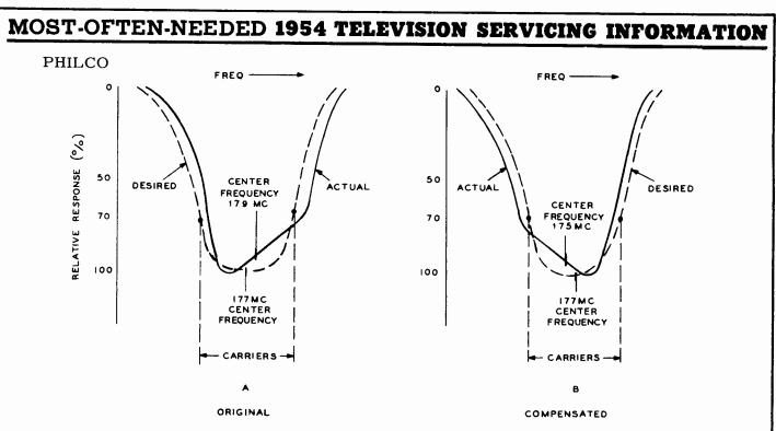
Figure 6. Television Tuner Response Curve, Showing Tracking Compensation
