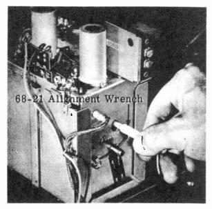
Fig. 11 Bulls-eye Tuning Adjustment.
