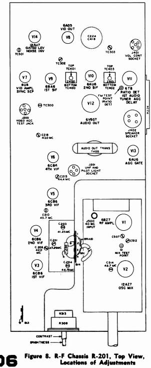
2. Tune the AM generator to 41.25 mc., and adjust C203 for minimum output, as observed on the oscilloscope.
