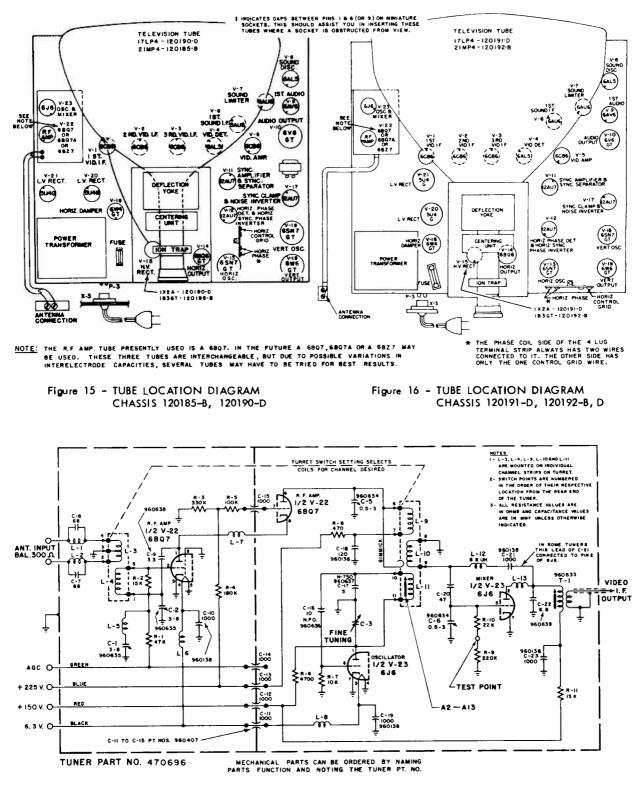
Figure 17 - SCHEMATIC DIAGRAM OF TURRET TYPE TUNER USED ON CHASSIS 120185-B, 120190-D, 120191-D AND 120192-B, D
