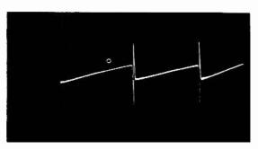
Vertical-Oscillator Plate, Pin 6 260 volts, 60 c.p.s.
