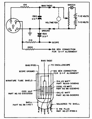
Figure 2. Video I-F Alignment Jig
