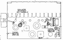
Figure 5—KRK12B Oscillator Adjustment
