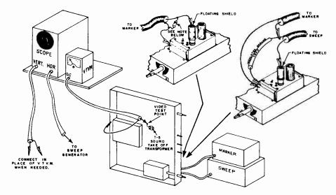
Figure 13. CONNECTIONS FOR I.F. ALIGNMENT.
