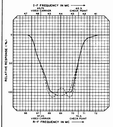
Figure 8. Over-All, R-F, I-F Response Curve, Showing Tolerance Limits
