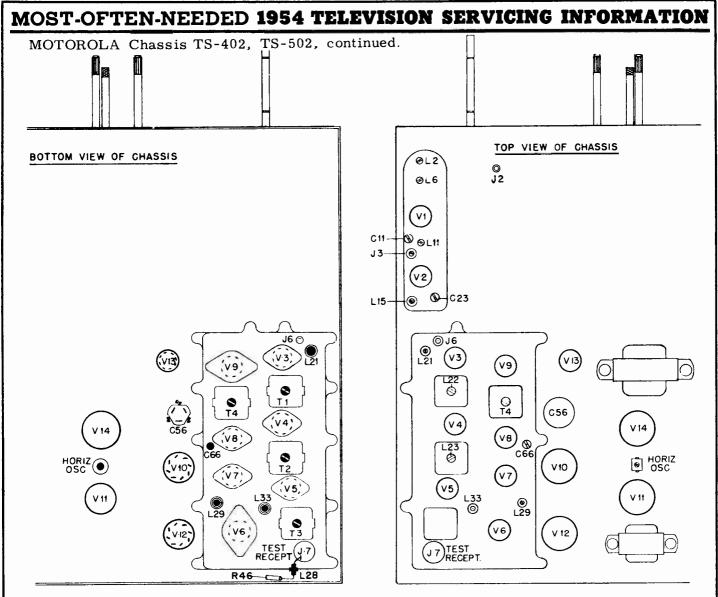
FIGURE 5. ALIGNMENT ADJUSTMENT LOCATIONS
