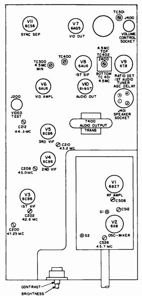
Figure 7. R-F Chassis R-191, Top View, Showing Locations of Adjustments
