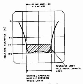
Figure 5. Television Tuner Response Curve, Showing Bandpass Limits
