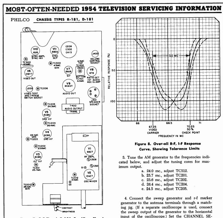
Figure 7. R-F Chassis R-181, Top View, Showing Locations of Adjustments
