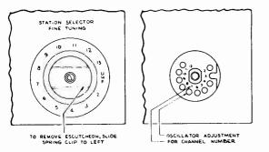
Figure 4—KRK29 R-F Oscillator Adjustments
