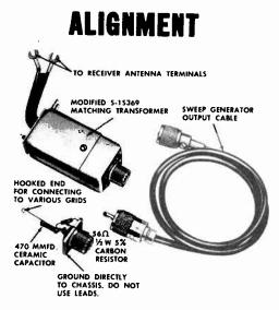
Fig. 15 IF-RF Alignment Fixtures
