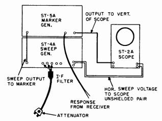
Fig. 15. I-F Sweep Equipment Connection Diagram
