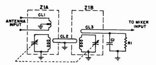
Figure 31. Equivalent Circuit of Preselector.
