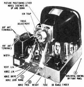
Rear View of VHF-UHF Chassis Showing Antenna Terminals and Adjustment Locations.
