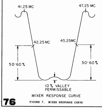
not change more than 0.2 mc. If the bandwidth does change more than 0.2 mc, check the cathode resistors, bypass capacitors, and tubes.
