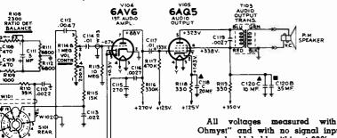
All voltages measured with "Volt-Ohmyst" and with no signal input. Voltages should hold within  $\pm 20\%$  with 117 v. a-c supply.
