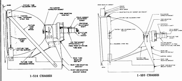
PICTURE TUBE INSTALLATION
