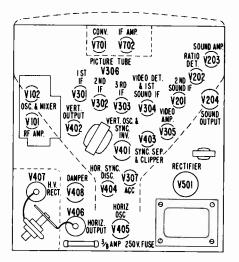
Top View of 22P2 Chassis. (V701 and V702 are accessible from underside of chassis.)
