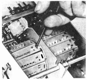
Fig. 13 Removing Channel Strips.
