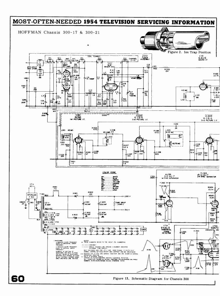
The source of protection which is provided in the chassis is the fusable resistor, R801. The entire receiver is protected against overloading due to short circuiting that results in excessive input current being drawn by the selenium rectifiers. R801 will open circuits on several times normal load.
