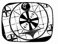
**Picture Tilted; Adjust Deflection Yoke Coil.**
