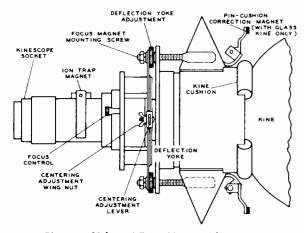
Figure 2-Yoke and Focus Magnet Adjustments
