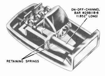
Figure 6. Top Inside View of S11A Son-r Tuner. Location of Retaining Springs and Resonator Bar Shown.
