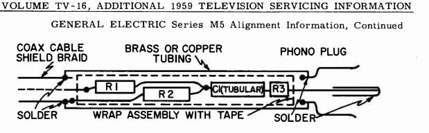
FIG. 3 I-F INJECTION PLUG CONSTRUCTION
