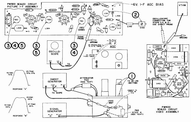
Figure 10-Sweep Alignment from Mixer Grid
