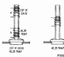
3. ADJUST... sound trap (L-107) to find the two points of adjustment at which the sound beat is just noticeable on the picture tube screen. Rotate the core toward center of the two points. Use minimum amount of inductance (core out of coil) that will result in no apparent beat interference.
