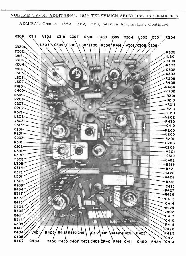
Figure 16. View of Components Side of Etched Circuit Board A7265-1. Location of Components Shown.
