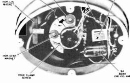
Figure 1. Adjustment Access Cover Removed - 9L38
