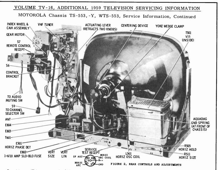
Do not turn oscillator screw counterclockwise to the extent of disengagement from tuner. To insure that the screw is within the range of its threads...tighten the screw (clockwise) until it stops, then turn counterclockwise until the station appears. The maximum number of safe counterclockwise turns from the stop are:
