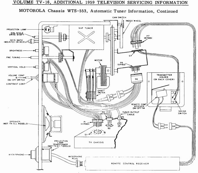
FIGURE 12. INTERCABLING & PLUG DESIGNATION DETAIL.
