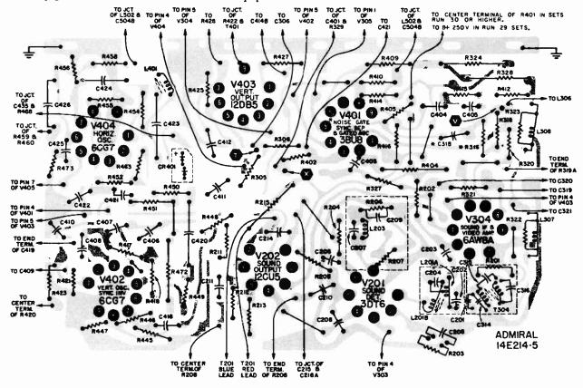
View of Printed Wiring Board A5780-5 used in 16R1, 16AR1, 16S1, 16AS1 Chassis. Note: Noise Gate Circuit in Chassis Stamped Run 30 or Higher. Gray Area Represents Printed Wiring; Black Symbols and Lines Represent Components and Connections on Opposite Side.
