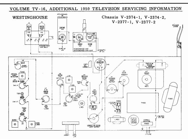
Figure 2. Top view of chassis showing tube locations, heater string, and adjustments.
