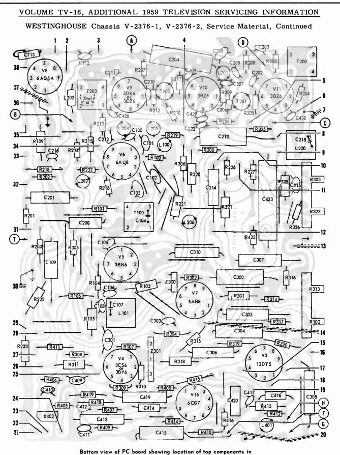
solid outlines. Tube pin numbering is for bottom of socket.
