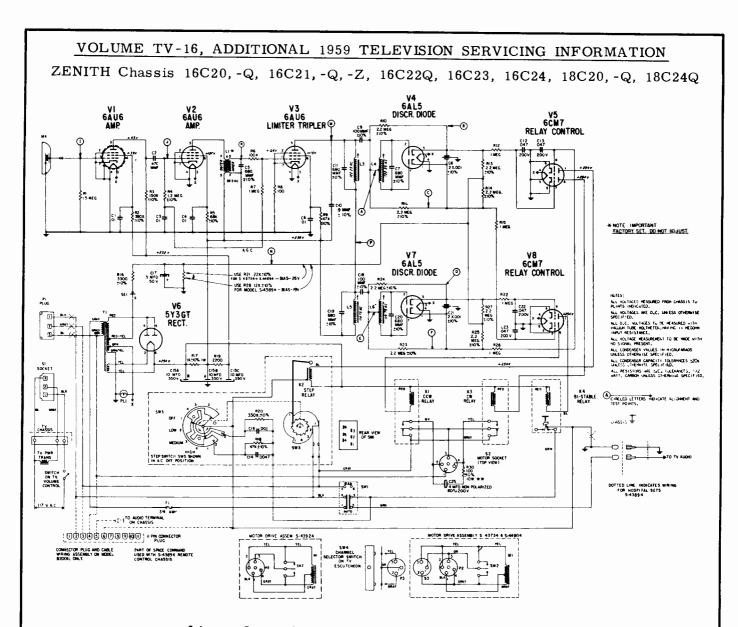
Schematic Diagram S-45834 Space Command Control Chassis
