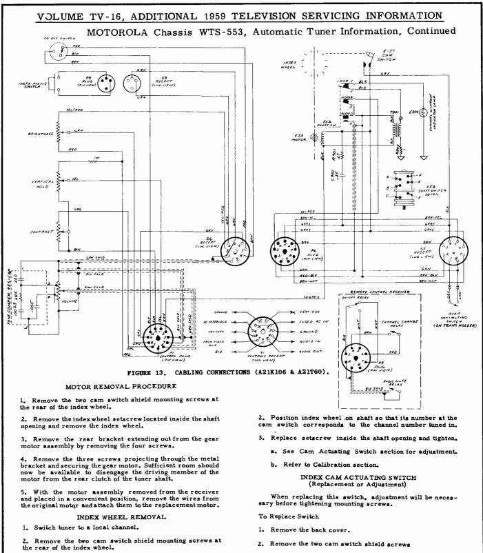
3. Remove the index wheel setscrew located inside the shaft opening and remove the index wheel.
