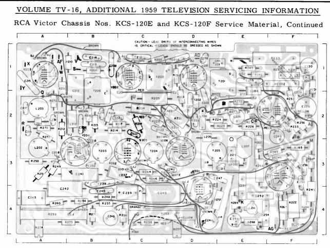
The printed wiring, on the reverse side of the circuit assembly, is presented in "phantom" view super-imposed on the component layout. This will enable circuit tracing without removing the assembly from the chassis to see the printed wiring on the reverse side.
