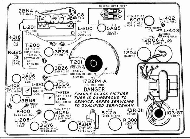
Chassis Tube Layout and Trimmers
