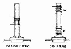
FIGURE 6. COIL CORE POSITIONS
