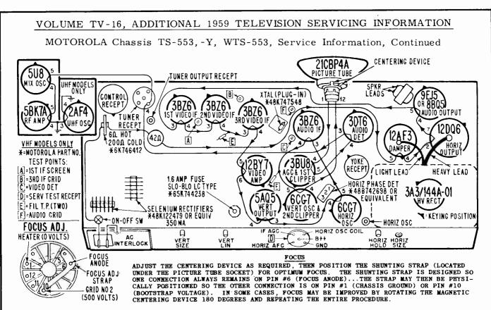
FIGURE 1. TUBE LOCATION, FUSE GUIDE, FOCDS INFORMATION & FILAMENT WIRING
