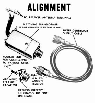
Fig. 4 IF-RF Alignment Fixtures
