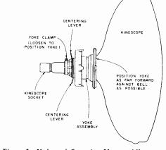
Figure 3—Yoke and Centering Magnet Adjustments
