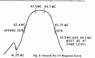
3. Set channel selector to Channel 13. Connect sweeper with very short leads through a 10 K mmf disc ceramic capacitor to mixer grid (lead of a 10 K resistor which is accessible through a hole located on front of the tuner). Readjust sweep output for 4.0V P-P, adjust 41.25 mc trap (bottom of L-200) so that notch is at marker, adjust mixer plate coil (L-9 primary) and input grid coil (top of L-200) for maximum gain and symmetry with 45.75 mc marker at 50%. (Figure 6.)
