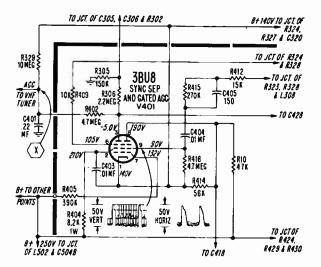
Sync Separator and Gated AGC Circuit Used in 16R1, 16AR1, 1651 and 16AS1 Chassis Stamped Run 29.
