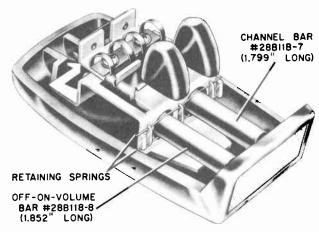
Figure 7. Top Inside View of S21A Son-r Tuner. Location of Retaining Springs and Resonator Bars Shown.
