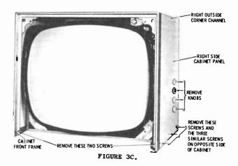
tighten into the outside corner channels shown in Figure 3C, which match the cabinet color. The cabinet-front-frame is secured to the corner channels by four (4) screws: two in each corner channel. (See Figure 3D.)
