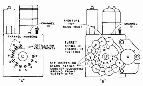
Figure 4-VHF Oscillator Adjustments
