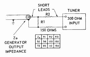
Figure 9. Impedance matching network.
