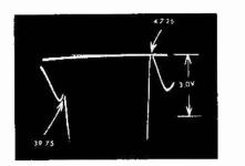
Fig. 7 Further Expansion of Fig. 6 for Detail View of the 39,75 and 47.25 Mc Traps.
