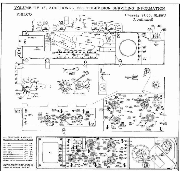
Chassis Layout Showing Voltage and Resistance Readings
