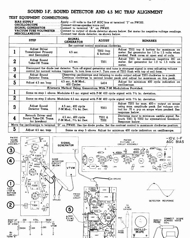
Figure 15-Sound I-F, Sound Detector and 4.5 mc. Trap Alignment
