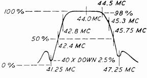
Fig. 5-Overall Response Curve
