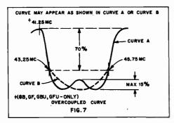
plus side to ground and minus side to junction of R14 and L3 (this point is AGC bias voltage) for all alignment procedures. Connect the marker generator to point illustrated in Figure 6 and set it to frequencies of 43.25 MC and 45.75 MC and connect the scope as shown in Figure 6. Alignment is done from the underside of chassis.
