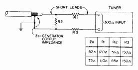
Figure 11 - Impedance matching network.
