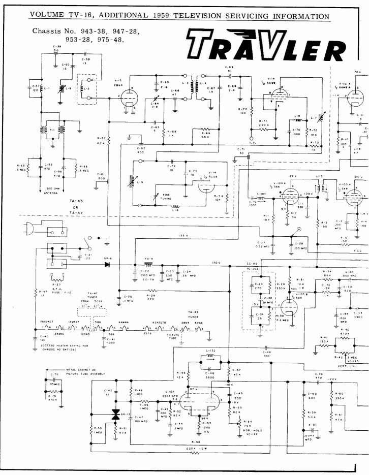
TRAV-LER RADIO CORP. Chassis Nos. 943-38, 947-28, 953-28, 975-48 Schematic Diagram, Additional Information on page 152.
