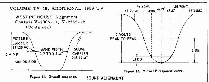
The sound section may be aligned using either a locally generated signal or an air signal.
