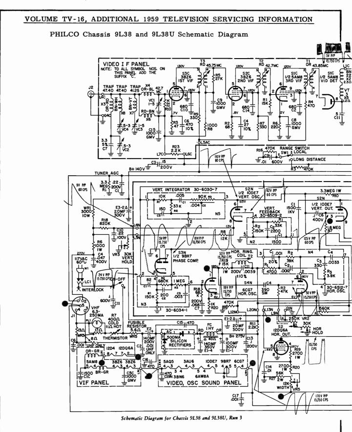
NOTES: All capacitor values greater than I are in MMF unless otherwise noted. All capacitor values less than I are in MFD unless otherwise noted. All resistors are 1/2 watt, 10%, carbon unless otherwise noted.
