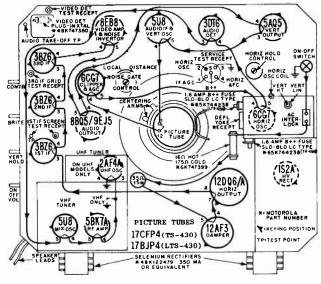
FIGURE 1. TUBE LOCATIONS & FILAMENT WIRING
