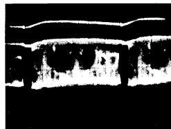
3 VERT. RATE 80 V P-P V201B PIN 9 VIDEO AMPLIFIER PLATE
