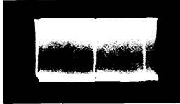
③ TP-5 SYNC PLATE VERTICAL RATE 60V P-P
