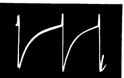
⑤ V206B PIN 9 VERTICAL OSCILLATOR GRID VERTICAL RATE 180V P-P
