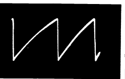
⑥ V206A PIN 2 VERTICAL OUTPUT GRID VERTICAL RATE 28V P-P
