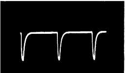
④ TP-5 SYNC PLATE HORIZONTAL RATE 60V P-P
