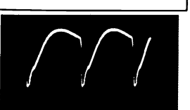
⑪ SR201 CATHODE JUNCTION HORIZONTAL PHASE DETECTOR HORIZONTAL RATE 12V P-P
