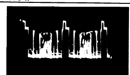
⑧ V205B PIN 9 VIDEO AMPLIFIER PLATE HORIZONTAL RATE 110V P-P
