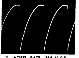
11 HORIZ. RATE 165 V P-P V101 PIN 6 HORIZONTAL OUTPUT GRID
