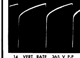
14 VERT. RATE 365 V P-P V502B PIN 2 VERTICAL OUTPUT GRID
