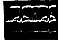
4 Volts p/p, 60 cps (max contrast)
