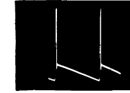
1000 Volts p/p total, 180 Volts p/p, sawtooth, 60 cps
