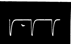
④ TP-5 SYNC PLATE HORIZONTAL RATE 60V P-P
