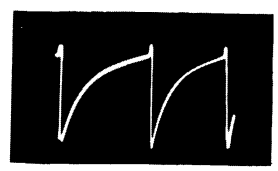
5 V206B PIN 9 VERTICAL OSCILLATOR GRID VERTICAL RATE 220V P-P
