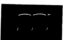
15 V105 PIN 2 KINESCOPE GRID HORIZONTAL RATE 40V P-P
