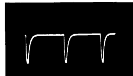
④ V201B PIN 1 SYNC PLATE HORIZONTAL RATE 60V P-P
