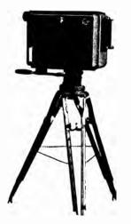
The modern type of camera as illustrated can be raised, lowered, and tilted automatically by means of electrical power. Inside the camera is housed the Iconoscope tube and is connected by means of cables to the associated amplifiers.
