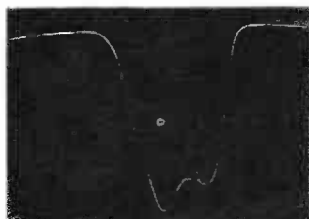
Figure 15-G Oscillogram of overall sound IF response. (The improper alignment is due to the different amplitude of the signal now being applied to the grids of each stage.) (Birdie at 21.9 mc.)
