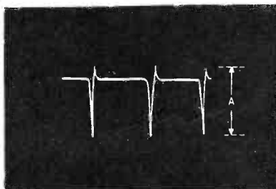
Sync Amplifier Grid Tube V2 Pin 1 A=4.5 volts
