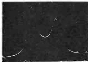
Figure 15-B Oscillogram of the single sound IF curve (untuned). This is the response curve appearing on the right of Figure 15-A after it has been expanded.
