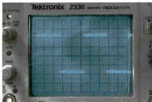
Figure 3 An internal graticule eliminates all parallax. Shown here is the probe frequency-compensation square waveform after the probe was calibrated correctly. The high brightness allows good viewing in bright ambient lighting, as pictured.
