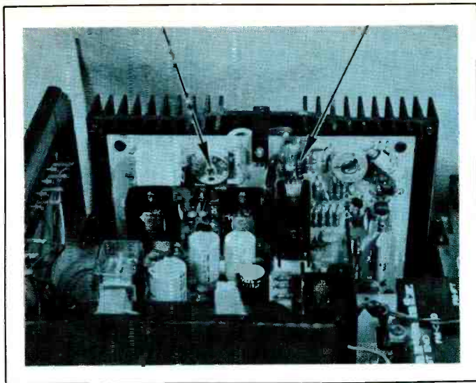
Figure 3 The left arrow on this picture of the right-channel circuit board points to R740 which was noisy and erratic. The right arrow shows where the two defective components were located. In the foreground is the small board containing the speaker-protection circuit, while the speaker terminals are at the extreme left.
