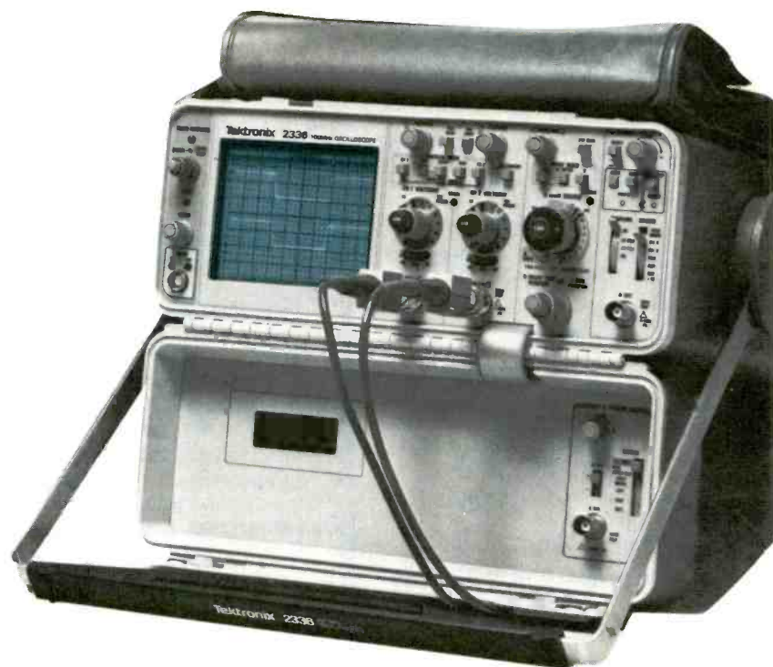
Figure 1 Tektronix model 2336 is a full-featured 100MHz portable scope. The hinged front cover locks in the open position (as shown) while the scope is raised by the handle. A plastic pouch for probes, books and tools is fastened to the top. Model 2336 was designed to resist hostile environments for field service.
