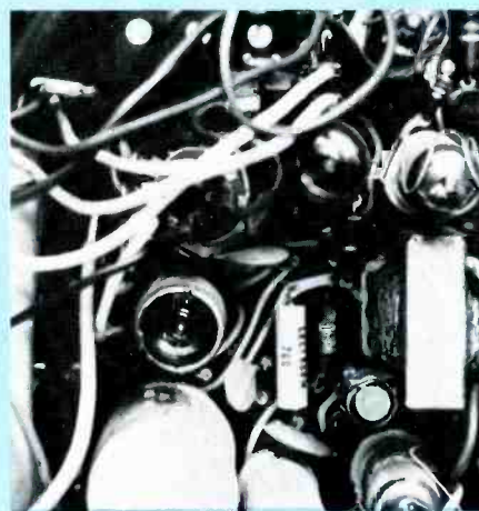
Figure 3 Several critical areas in older 500-series Bell & Howell projectors are identified here. Left, the arrow to the center locates the important worm gear (the one needing special-purpose grease). The tube-equipped audio board is pointed out by the arrow at lower right. Right, this closeup photograph shows the audio board, which is located below the motor in 500-series machines.
