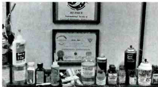
Figure 2 Many types of greases, lubricants and chemicals are required for servicing mechanical and electronic machines. Left, lubricants for most applications do not require critical specifications. However, for Bell & Howell 16mm projectors, these two greases are essential. At the left is Bell & Howell number 070034, a general-purpose grease. Notice the lack of shine. Number 070043, at the right, is a special-purpose grease for all plastic worm gears. It does not harden with age (notice the shiny surface). Do not substitute this grease with anything else, if at all possible. Right, many other chemicals and lubricants of less critical characteristics are needed.
