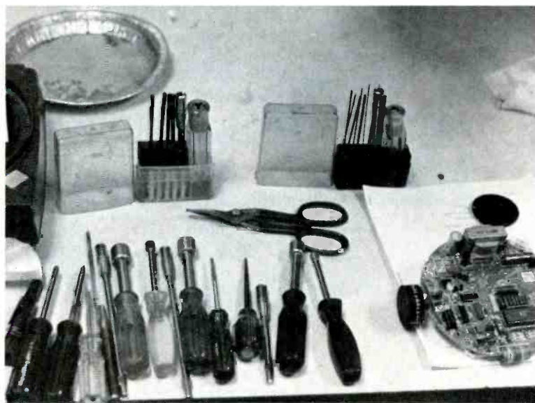
Figure 1 A wide assortment of tools is required for servicing audio-visual equipment. Left, this tool case with its tools is taken on regularly scheduled calls to schools all over the county. Below, another set of tools is kept at the repair shop in a central location.
