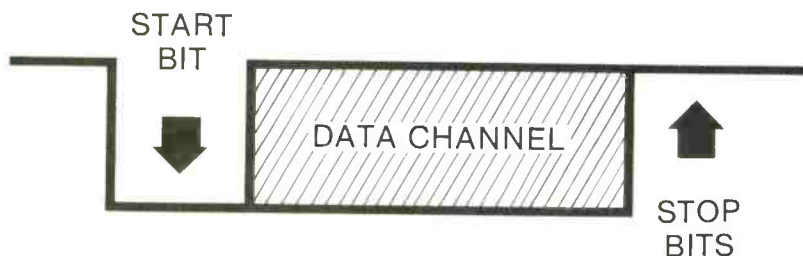
Figure 8. Serial data are clocked into a serial analyzer either synchronously or asynchronously, one bit at a time.
