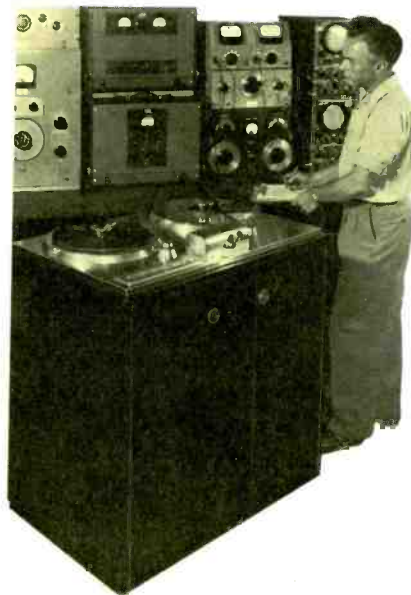
Ampex's Harold Lindsay is shown checking out a model 200 in late 1947. Note the Dumont scopes to his right, as well as the Altec intermodulation analyzers and Hewlett Packard VTVMs and signal generators. (Photo courtesy of Ampex Corporation.)
