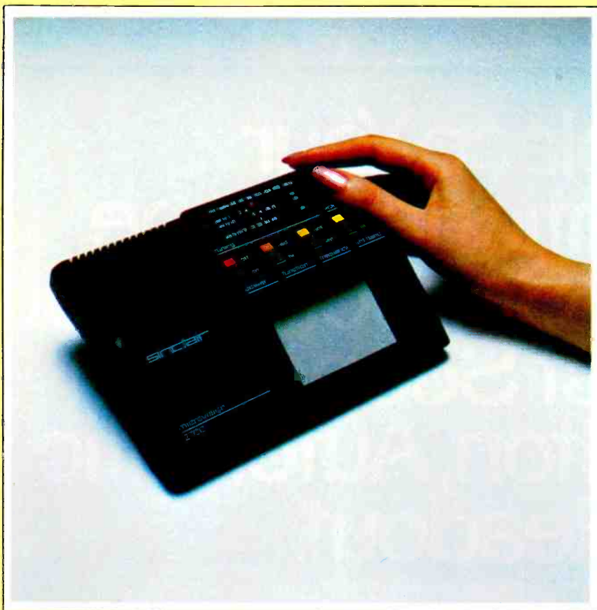
The deflection system that bends the cathode beam through 90 degrees makes a flat screen possible.
