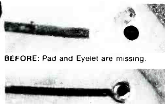
AFTER REPAIR with SRS-050 Kit, the Pad and Eyelet have been neatly replaced.
