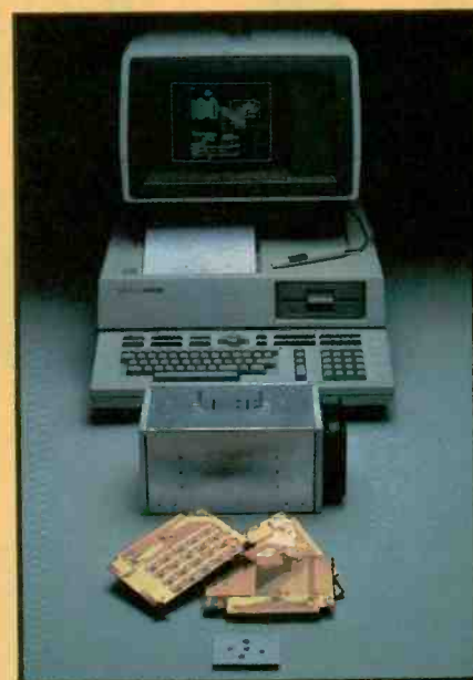
The five superchips in the foreground are the nucleus of each model in the HP 9000 family. The chips are mounted on boards that fit into a lunchpail-size module, which in turn is the basic power package inside the computer.
