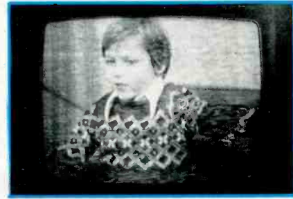
Figure 3. Drop-outs remove the video from one or several horizontal scanning lines on the TV receiver screen.
