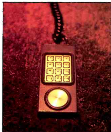
Figure 8. The hand controller is the player's input device to the game.
