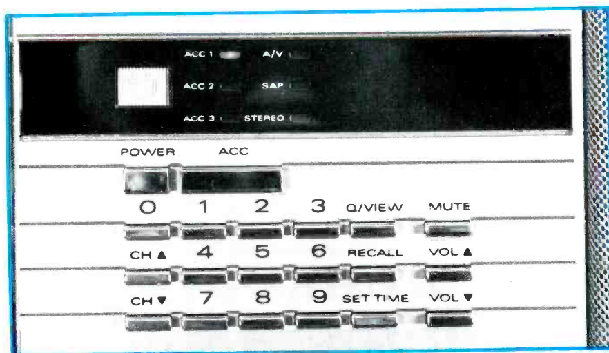
Figure 3. Some details can be seen of the sensor/indicator-light area above and the 20 push-buttons below.
