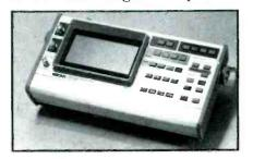
This mini oscilloscope uses four regular D-size batteries, or operates on an external ac adapter. Alphanumerics in the LCD screen indicate the peak-topeak voltage value, period and dc component. Screen size is approximately  $5^{1}/_{2}$ " x  $3^{1}/_{2}$ "; the cursor allows VPP time measurements with Delta time.
