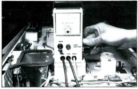
Figure 2. A defective magnetron may be detected by taking voltage and current measurements with the microwave oven Magnameter.
