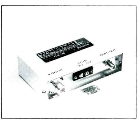
**Figure 5.** Voltage tunable, single-channel downconverter showing input (4GHz) and output (70MHz) connectors plus dc power cable connections.
