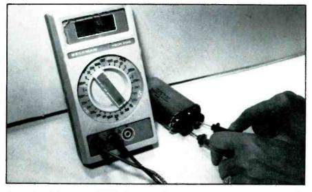
Figure 4. In this Norelco MCS7100 oven, only  $105\Omega$  were measured between the HV capacitor terminals. A normal capacitor will have infinite resistance.
