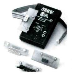
provides the lab or field technician with a quick-check method of determining whether a particular cable is basically good, possibly eliminating the need for troubleshooting a complete system.
