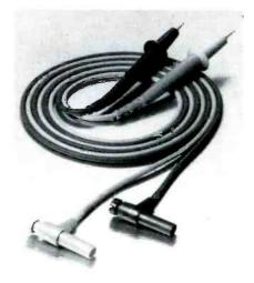
that expands the banana plug inside the meter jack for a tight connection. Banana plugs are rubbershielded for maximum safety. To minimize thermal EMF and contact resistance, contacts are silver plated. Ratings are 1000Vrms and 10A continuous current.
