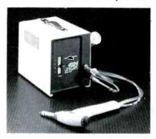
electronically controlled, variabletemperature for either soldering or desoldering is presented by the Ungar Division of Eldon Industries. Plug-in soldering and desoldering handles give the user the options of soldering or desoldering. Temperature can be set on a sliding scale from  $450^{\circ}$  to  $850^{\circ}$  F. In the soldering mode, either a micro-sized or macro-sized soldering iron can be used; twelve standard Ungar tips are available for each.
