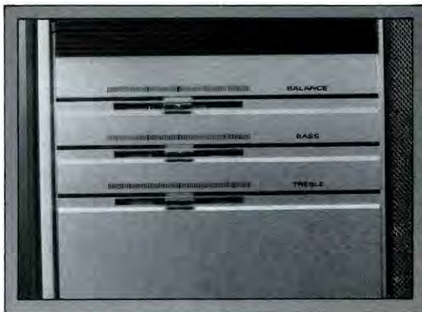
For the balance, bass and treble controls, neutral position is obtained with the dent in the bar knob vertically aligned with the black calibration line above it. Operations of the bass and treble controls are critical around the center or neutral position because the controls do not have a center tap on the element. Instead, it appears the boost and cut operations are in opposition at the center, making the point of cancellation very critical.
