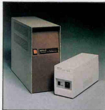
Standby power sources (SPS) provide clean, regulated ac power to critical loads when ac power fails or drops 15% below nominal. SPS units are available with outputs from 1,200VA down to 300VA.
