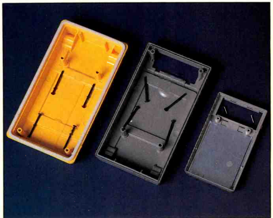
Shown left to right are the bottom cases of three DMMs. The major factor of mechanical protection is case design, including the number of internal ribs supporting the case, thickness of the material and number of screws holding the case together. For protection from contaminants such as water, a gasket is needed, as shown in white on the yellow heavy-duty meter.
