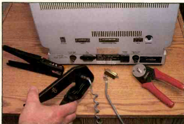
In this application, an 8-position silver satin line cord must be stripped and, depending on the hardware, a DB-25 or RJ-45 connector must be installed.
