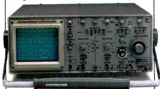
Model 9106, 60MHz, 3 Channel, Dual Sweep (A & B).
