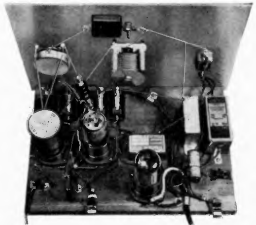
How the two-tube set on page 10 should look after adding a stage of audio amplification
