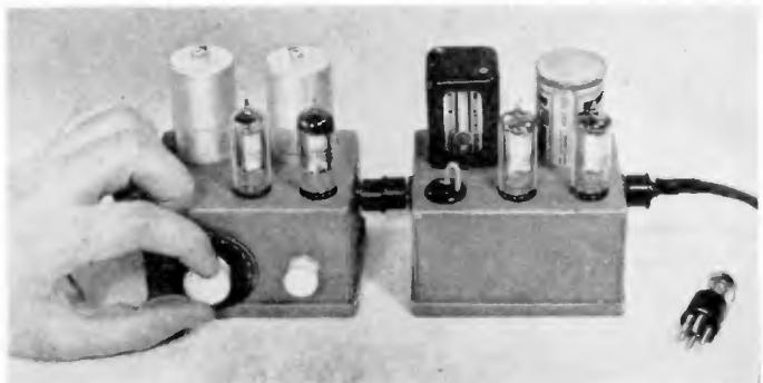
At the left is the tuner unit. It may be used individually as a headphone receiver or with the amplifier as a broadcast set
