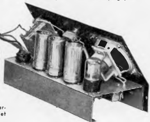
Keep tuned as you ride with this receiver. Note below how tubes are mounted on aluminum chassis, and the speaker on the sloping panel
