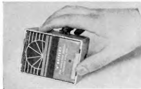
The 67 1/2-volt "B" battery that supplies plate current to all the tubes in the two units fits snugly in the bottom of the gray wrinkle amplifier cabinet
