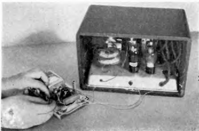
An ordinary bell transformer furnishes the heater supply. At left, hooked up and ready to go, showing its small size
