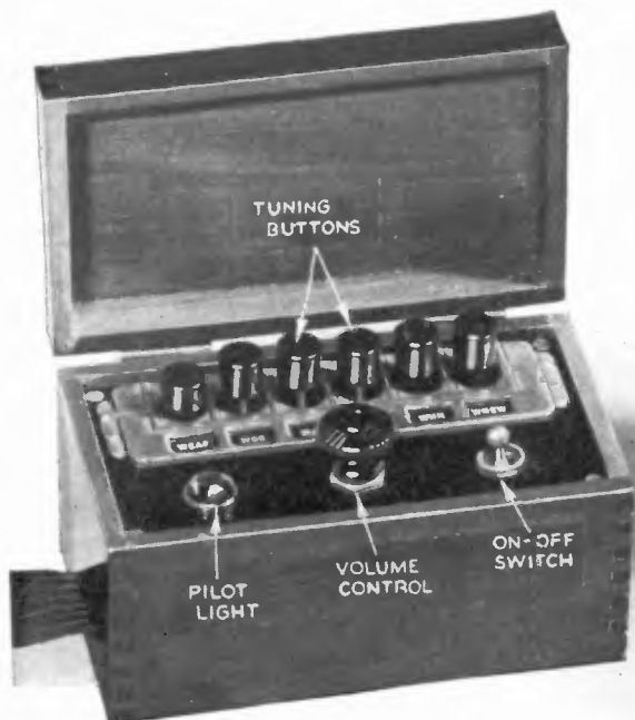
The push-button case also houses a volume control, an on-off switch, and a pilot light. Brackets aid in mounting the relay unit
