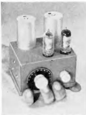
At the left is the tuner unit. It may be used individually as a headphone receiver or with the amplifier as a broadcast set
