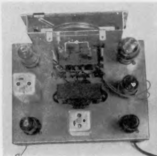
Top and bottom views of the chassis show how "permeability tuning" saves space, eliminates crowding, and simplifies wiring of the circuit
