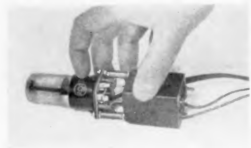
Illustrating how to make a compact "batch" of the condenser and resistor in rectifier, with connections
