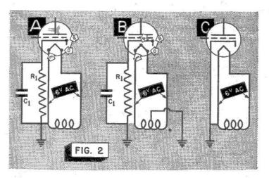
if the capacity is insufficient, or if there is a considerable amount of amplification between the grid circuit of this stage and the output, even a small amount of hum voltage developed across  $R_1$  will be amplified sufficiently to cause hum.
