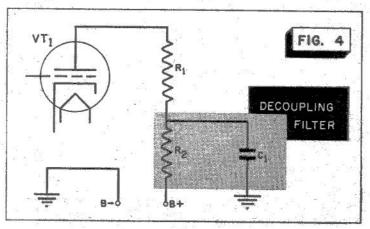
will first have to use the methods described later to determine which stage the hum enters. Then you can try moving the leads in that stage with an insulated stick or alignment tool while the receiver is turned on. If you find a position where the hum disappears, you have solved the problem. Examine the set carefully to see if there is any evidence of shields missing. Also, if the control grid lead should be brought up inside a shield, be sure it is so placed.
