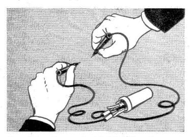
The easiest way to connect a test electrolytic condenser across a filter condenser is to clip test leads to the terminals of the test condenser, as shown above, and touch the prods on the other ends of the leads to the terminals of the filter condenser. CAUTION: Be careful not to let your fingers touch the power supply circuits—you can get a severe shock.
