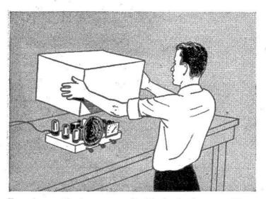
To make a set heat up on your bench, simply place an ordinary cardboard box over it. Make sure the box is large enough to rest on the bench all around the set.
