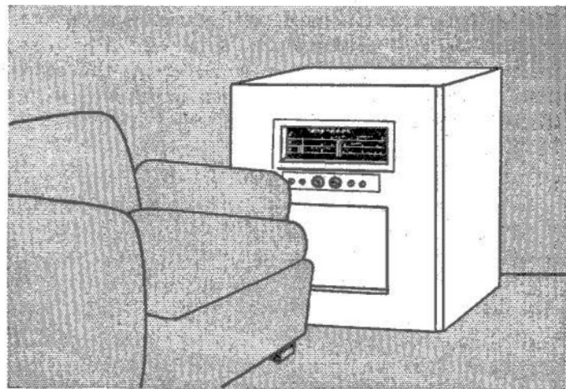
If the customer complains that the tone of his receiver is not clear, make sure the set is not placed so that a large chair or other piece of overstuffed furniture is close to it and directly in the path of the sound waves produced by the loudspeaker. The chair will tend to absorb high frequencies, creating a muffled sound.
