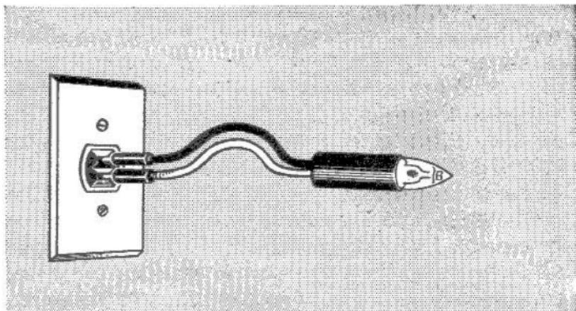
When a set is completely dead, always check the wall outlet to make sure it is "hot." A neon test light like this one is a handy device for testing the outlet. If you prefer, you can plug in a lamp or use your voltmeter to make the check. If you find no voltage at the outlet, most likely a fuse is blown in the power line.
