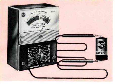
One of the major service aids that are part and parcel of the 1959 RCA battery program is the WV-37B Battery Tester, an accurate, attractive, and highly flexible instrument.
