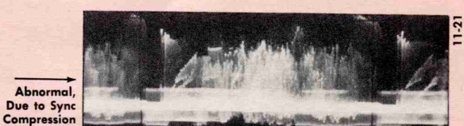
6J. Another example of the trouble shown in 6I. This condition results in unstable sync action, or loss of sync.
