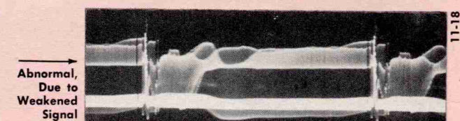
6H. If for any reason the amplitude of the TV signal at the input to the sync separator is considerably lower than normal, the output will be distorted and will vary with changes in picture content.
