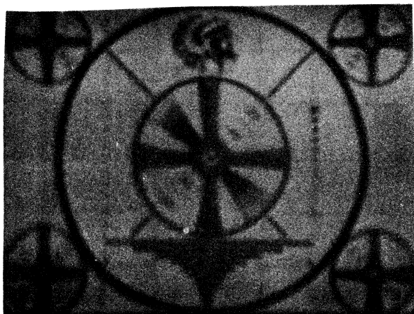
FIG. 4.—Focus control misadjusted: The whole pattern becomes fuzzy and except at the outer edges there has been a graying of the entire pattern.
