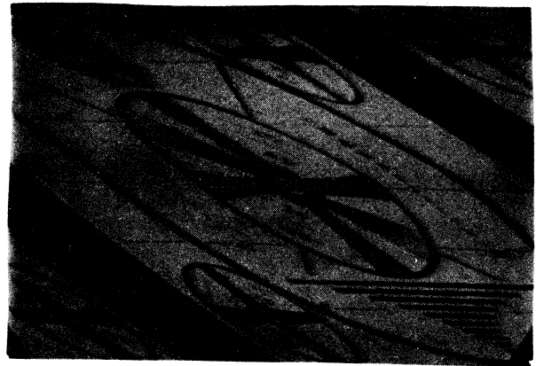
FIG. 8.—Horizontal hold control misadjusted: The test pattern leans to right or left on the screen.
