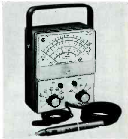
Fig. 1 RCA VoltOhmyst, Model WV-500A, solid-state electronic VOM.
