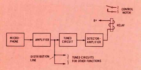
Fig. 4 Block diagram of a typical remote receiver.
