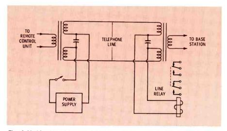
Fig. 4 Modification of grounded remote control system in Fig. 3. System shown here is ungrounded, which eliminates ground currents and their effects.
