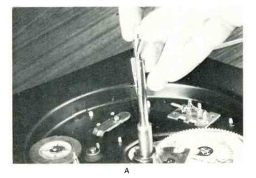
Fig. 4 Record-dropping assemblies. (A) Spindle has spring, pushrod, and push-off tab; also has guides to keep record stack in position. (B) Link from cycling slide has drop-slot at left end to engage spindle pushrod. (C) Push-off tab in position to push off record.
