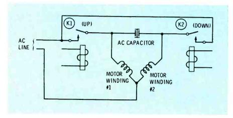
Fig. 6 Circuitry of two-phase motor used to remotely control volume, tint and color saturation.
