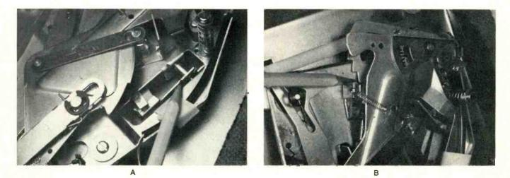
Fig. 6 For indexing at automatic shutoff, (A) record-support arm pushed trip pawl out of way. Indexing bar snaps all the way back and (B) stops tone arm swing by catching last serration.
