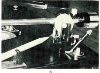
Fig. 2 Assembly that raises tone arm. (A) Pencil points to small spring that encloses pushrod, which rests on bent tab of cycling slide. (B) Small platform pushes upward on adjustment screw. (C) Cue lever lets you raise tone arm manually.
