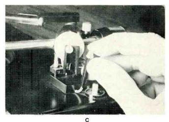
Troubles with dropping are more often in the spindle than anywhere else. The spring for the push-off tab gets weak. The tab and pushrod may get sticky, particularly if some misguided soul tried to oil them. Or the tab gets bent. Or the guides get sticky. The cure is a new spindle -usually inexpensive.
