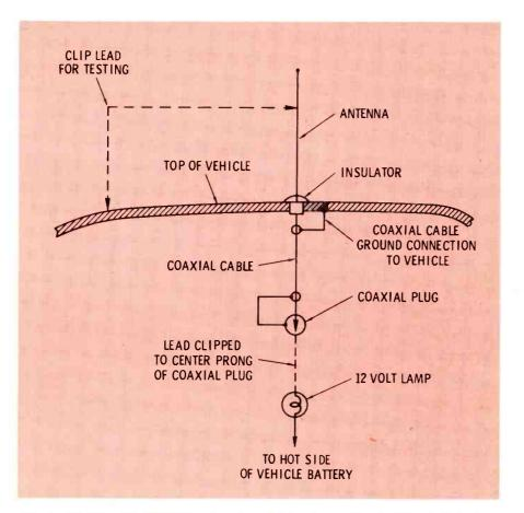
**Fig. 1** Test setup for checking out a whip antenna not equipped with a built-in shunt impedance matcher. Ground the whip to the body of the vehicle and connect a test lamp between the "hot" lead of the coax and the 12-volt battery of the vehicle. If the lamp lights, the antenna is not open. If the lamp remains lighted after the antenna-to-vehicle test lead is removed, the antenna or coax is shorted.
