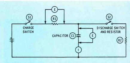
Fig. 2 (A) Schematic of the circuit used to chart the charge and discharge of capacitors.
