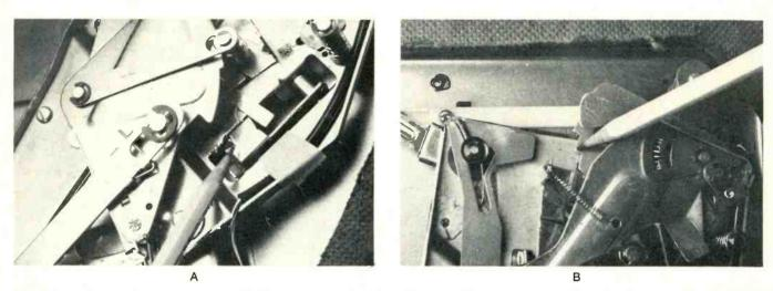
Fig. 5 Indexing mechanism consists of (A) blocking tab and indexing bar. (B) At other end of indexing bar, serrations in tonearm lever catch on index-bar tab, preventing tone arm from moving further inward than lead-in groove of record size chosen.
