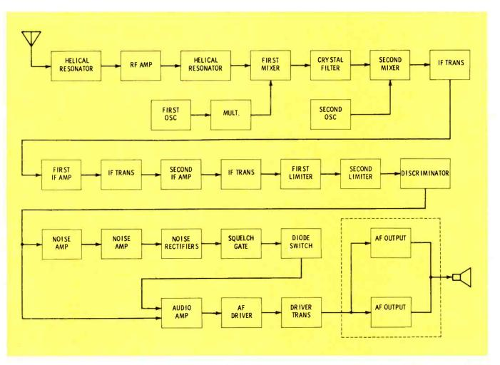
Fig. 5 Block diagram of a typical FM communications receiver. Compared to a color TV receiver, it is relatively simple. (Courtesy E. F. Johnson Company)
