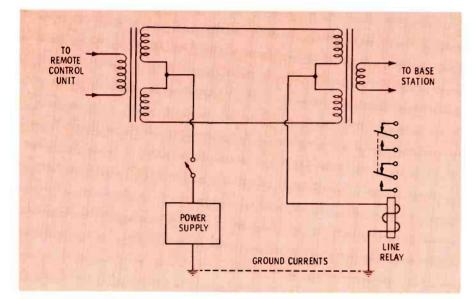
Fig. 3 Ground currents (indicated by dotted line) caused voltage across line relay to vary, causing the transmitter to operate intermittently. System shown here is a simplexed-to-ground remote control system.
