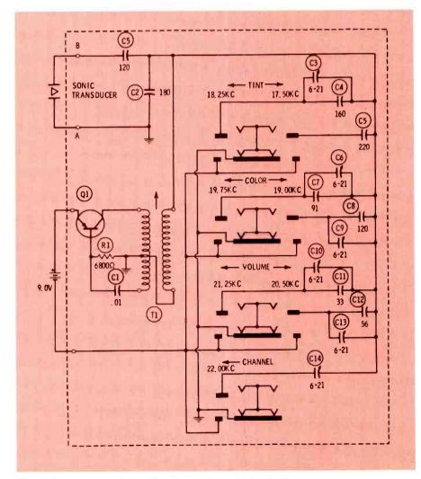
Fig. 1 Remote transmitter with a trimmer for each frequency.
