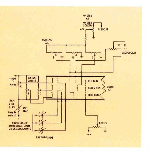
Fig. 1 Simplified schematic of various color-CRT control circuits. No single set has all these controls, but positions and relationships to other circuits are shown here. Control labels vary with chassis, too, and the most popular are listed.
