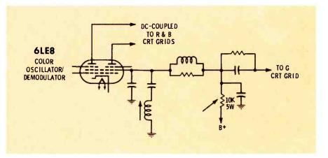
Fig. 3 Special tube oscillator/demodulator for color might fool you if you're not familiar with the stage. But that needn't keep you from tracing down DC trouble that puts a gray-scale symptom in the raster. Just start at the CRT and work back.
