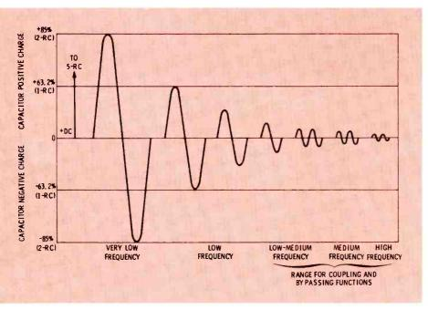
Fig. 3 If the supply voltage is changed to AC, the amount of charge the capacitor accepts is determined by the frequency of the AC.
