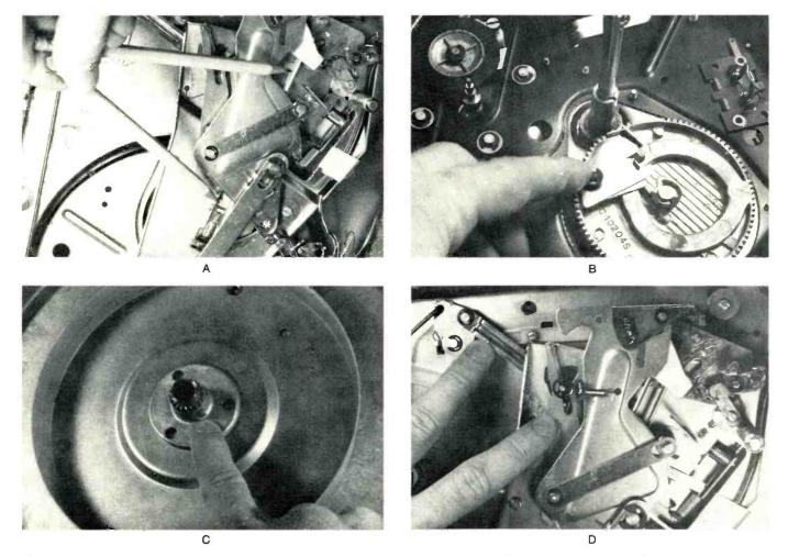
Fig. 1 Tripping mechanisms that initiate change cycle. (A) Pencil points to sliding linkage that is actuated by lever on bottom of tone-arm pivot. (B) Jointed trip pawl is part of cycling gear. (C) Cast-metal tab on hub of turntable catches trip pawl to start change cycle. (D) These linkages move trip pawl from reject lever.
