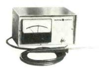
control of tip temperature, and an adjustable set-point circuit that provides full-power response to load in seconds. It operates in the 100- to 1000-degrees (F) range.
