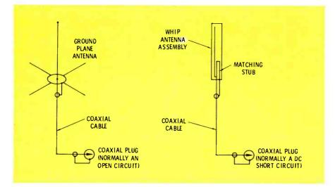
**Fig. 2** Whip antenna equipped with a matching stub normally indicates a dead short when checked with an ohmmeter; ground-plane type on left normally indicates an open circuit.
