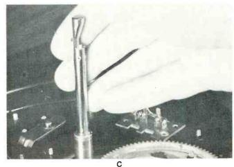
full circle. The cycling slide is moving back to its beginning position. As it does, the bent tab moves back from under the arm-lift pushrod and platform. The platform lowers to its resting position. If indexing is correct, the needle sets down in the lead-in groove of the record that just dropped.
