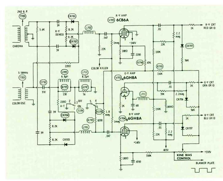
Fig. 1 Complete schematic of the demodulators and color-difference amplifiers in the new RCA CTC39X chassis. Notice especially the circuits connected to switch S106, the Accu-Tint OFF/ON switch.
