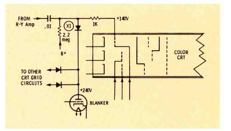
Fig. 2 DC restorer, or clamper, helps maintain proper DC level on CRT grid. A shorted or leaky diode can alter gray scale of the CRT raster.
