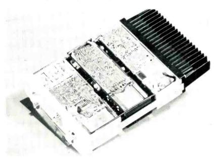
Example of a solid-state mobile communications unit employing printed-circuit boards.
