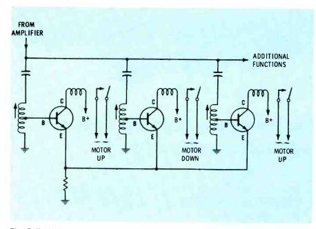
Fig. 5 Typical remote-receiver output circuits.
