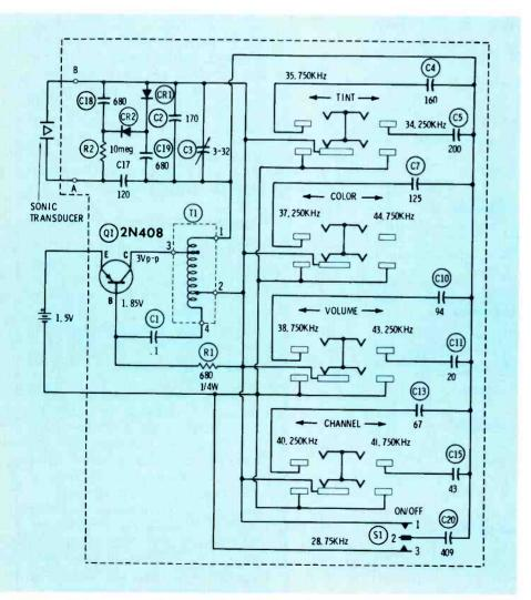
Fig. 2 Remote transmitter with a single tuning adjustment.
