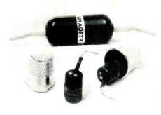
metal shields, the transformers come in two types: Model BV-16 is rated at 200 to 50K ohms and is mumetal encased for chassis mount. Model BV-16E is electronically identical to Model BV-16 and comes encapsulated in vinyl, with an 8inch length of microphone cable. Model BV-16E can be installed in or out of the microphone case, or it can be installed in the line.
