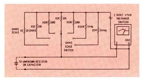
**Fig. 8** Schematic of a typical ohmmeter function in a VTVM or FET meter. Connect the ohmmeter leads to a capacitor and notice the similarity of this circuit and the diagram of the capacitor charging circuit in Fig. 2A. This similarity is the basis for a very simple method of measuring with an ohmmeter the capacitance of most electrolytic capacitors.
