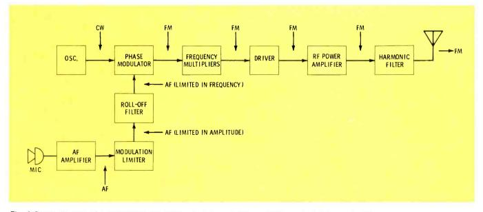
Fig. 6 Block diagram of a typical FM transmitter. It, too, is relatively simple compared to a color TV.
