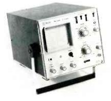
width, sensitive to 2mV/Div. The signal-derived triggering is automatic over the entire nominal 10-MHz bandwidth.
