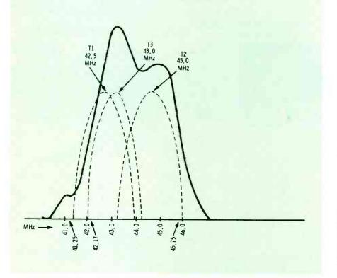
Fig. 5 Individual responses of stagger-tuned IF transformers combine to form IF response curve. Heavy line is the net response traced at all frequencies in the IF passband. It is the same curve you see traced by the sweep generator and scope in Fig. 3B.
