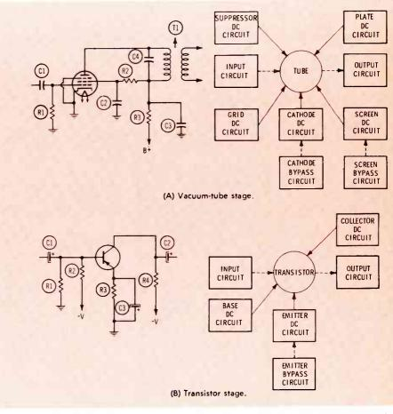
Fig. 3 Circuits in typical amplifier stages. Other signal circuits include feedback circuits, tuned circuits. Bypass circuits are often called decoupling circuits.
