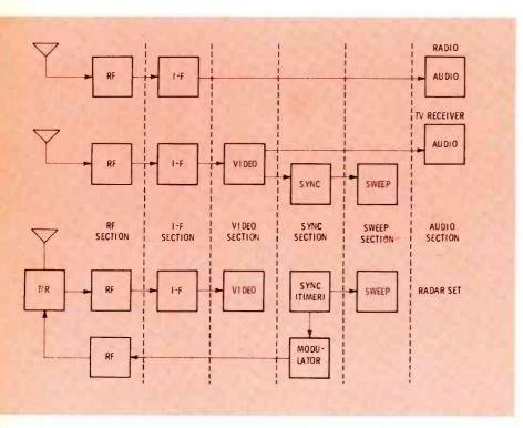
Fig. 1 Sections are the largest division of electronic equipment. Each section handles one kind of signal. When the nature of the signal changes, it's handled in a different section.
