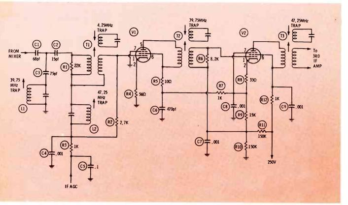
Fig. 4 Part of stagger-tuned IF strip that is used in many TV brands and models. This one is "B+ stacked" version, in which two tubes are in series across B+ line. Cathode and grid of V2 have high positive voltages.
