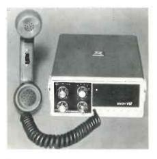
ing. A plug-in power lead is provided for easy removal and safekeeping. Also incorporated in the unit is a press-to-talk telephone handset and low-power switch.
