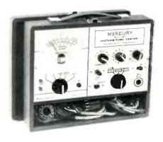
Model 880 contains universal sockets and adapters, including complete black-and-white sockets. Mercury states that each gun of a color tube is adjusted to cutoff before the beam current reading is taken, to simulate actual conditions in the television set. It also checks shorts or inter-element leakage.
