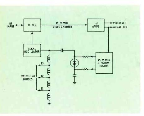
Fig. 3 The basic automatic-fine-tuning (AFT) loop.
