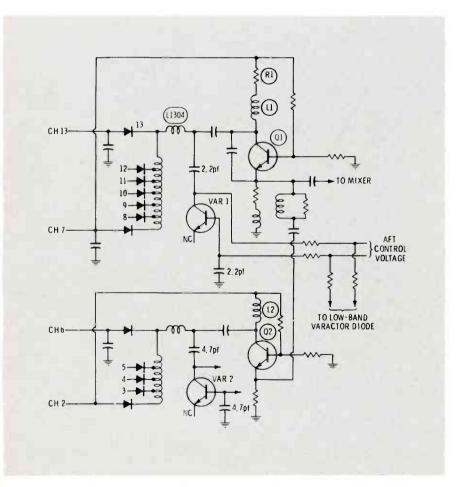
Fig. 4 The dual local-oscillator configuration, which is necessary to insure optimum AFT performance on all channels.
