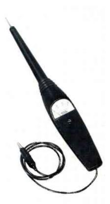
The HVP-5 reportedly measures voltage up to 30,000 volts with complete safety, and because it has a built-in voltmeter, eliminates the need for additional bulky equipment. Special barriers isolate the high-voltage tip from the probe handle and meter.
