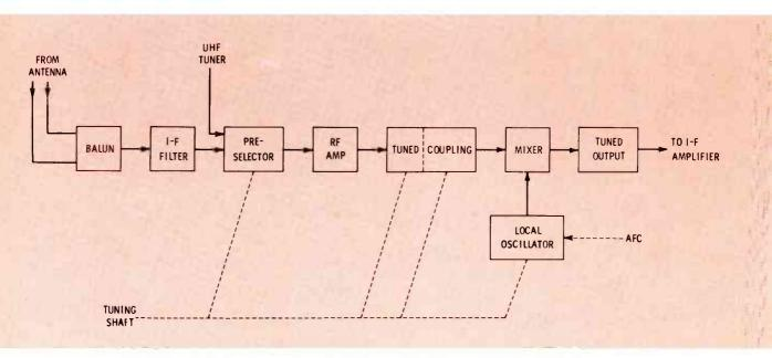
Fig. 1 Location of the tunable circuits in a typical conventional color television tuner.
