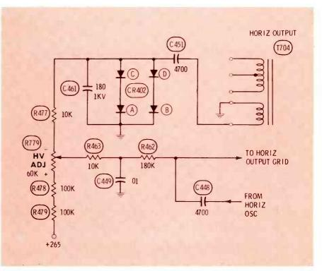
Fig. 14 To help insure adequate high-voltage regulation regardless of failure, four diodes are wired in series-parallel in the high-voltage regulator of Admiral's 19H10 chassis.
