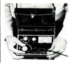
output which can be used to drive a high-impedance crystal earphone, a tape recorder or an oscilloscope. The unit automatically turns off when the cover is closed.
