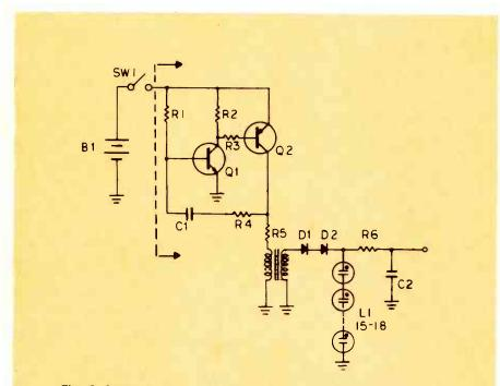
Fig. 3 Oscillator high-voltage supply employed in circuit design shown in Fig. 4.
