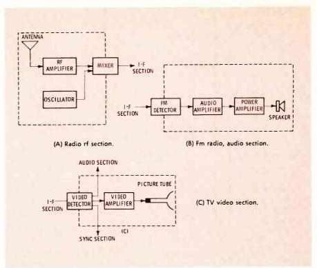
Fig. 2 Examples of how sections are divided into stages. Interface stages are the ones that change the signals, in preparation for feeding the signal on to the next section.
