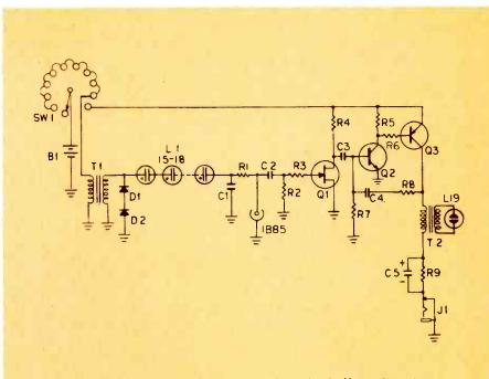
Fig. 1 Circuit diagram of circuit No. 1, a simple X-ray detection instrument.
