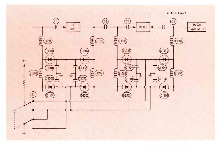
Fig. 2 Partial schematic of the electronically controlled tuner, showing the components for channels 12 and 13. An additional set of diodes and capacitors is used for each of the other channels.
