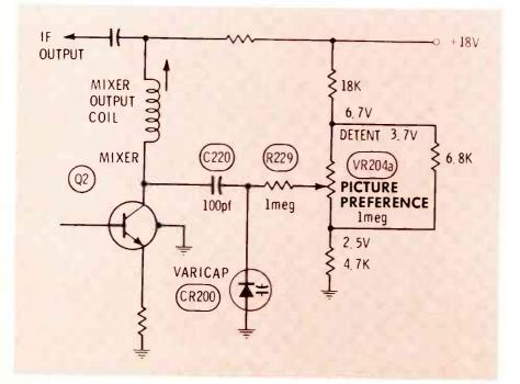
Fig. 8 A slight change of IF alignment by varicap tuning in the Philco 21ST90 chassis gives an effect similar to video peaking.
