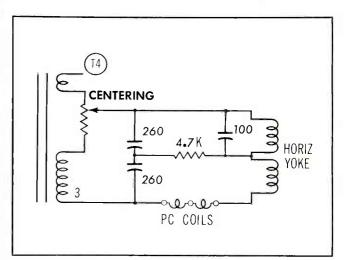
During normal operation, the two 260-pf capacitors (see diagram) and the two horizontal yoke windings form a balanced bridge. No voltage appears across the 4.7K-ohm resistor, except for a slight unbalance, and the resistor operates with very little heat.
