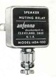
capsulated in the case to prevent malfunctioning from transmitted vibration. Also, the unit is hermetically sealed in a cadmium-finished case to prevent moisture seepage internally, rust externally. Maximum power is 5 watts continuous, and load resistance is 4 ohms.
