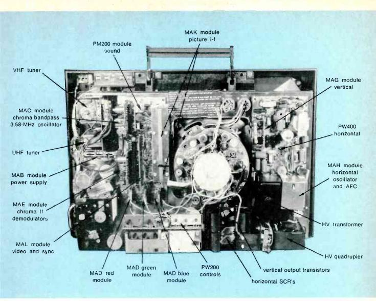
Fig. 11 Photo showing location of major components and the eleven modules that comprise the RCA CTC49 chassis.
