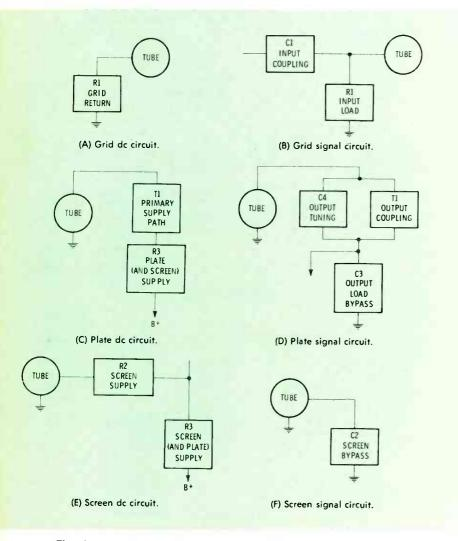
Fig. 4 Parts, the smallest division for 1-2-3-4 Servicing, often serve in more than one circuit. Examples are shown here for both signal and DC circuits in Fig. 3A.
