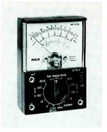
from 0.2 to 600 volts, in four ranges; DC current from one microampere to 300 milliamperes, in three ranges; and resistance from one ohm to five megohms, in three ranges; and decibels from -20 to +37.
