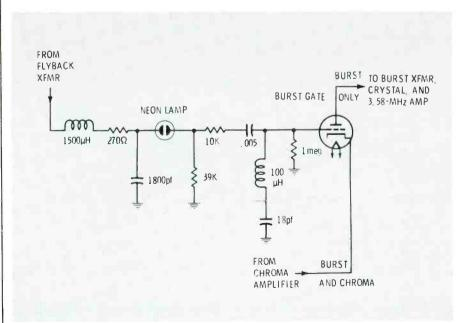
Fig. 4 Burst-gate stage in GE chassis has neon lamp input clipper. If the lamp doesn't fire, burst doesn't get through the triode. Without burst applied to the color-subcarrier amplifier, the demodulators can't produce color.
