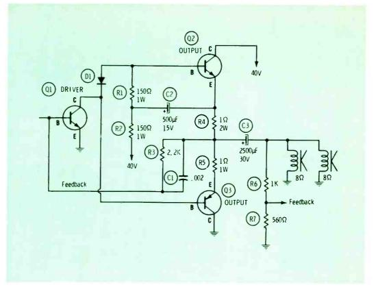
Fig. 3 Complementarysymmetry output stage draws its name from opposite-polarity transistors, which complement each other and drive speakers push-pull, without a transformer.
