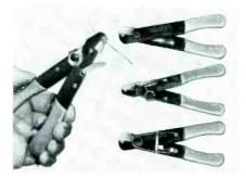
spring-equipped, self-opening handles. A slip ring holds the handles closed when not in use.
