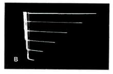
Fig. 6 If you can find two transistors whose characteristic-curve traces coincide, you can be assured they match dynamically. Traces shown here were produced by A) a 2N411 PNP germanium and B) a small NPN silicon.
