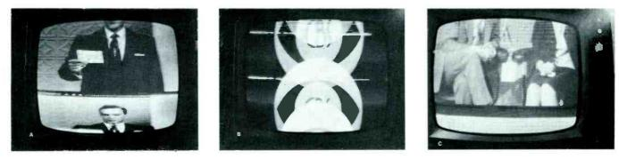
Fig. 1 Correct locking involves more than just stopping the picture from rolling—both frequency and phase must be correct. A) Sweep frequency of 30 Hz produces two complete pictures with the vertical blanking bar between them. B) Sweep
