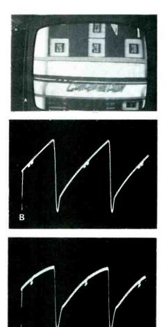
Fig. 4 Signal injection, using a 6-volt AC sine wave from the heater circuit in series with a .47-mfd capacitor, is an effective test. A) Picture obtained when the sine wave is injected at the grid of the oscillator. The picture continuously rolled down slowly. B) Waveform at the plate of the oscillator. Overload produces a waveform similar to that required. C) Waveform at the yoke; the voltage was 45 volts PP.
