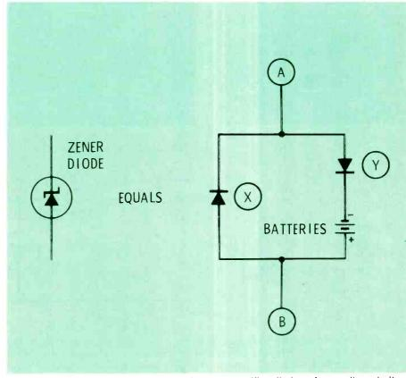
Fig. 3 A zener diode can be visualized as two rectifier diodes of opposite polarity connected in parallel, with a battery, used to provide a voltage delay, in series with one of them. Conduction can be obtained in either polarity, but at different voltages.
