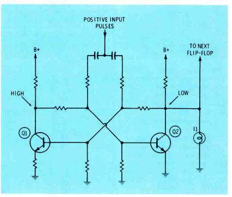
Fig. 1 The basic flip-flop multivibrator.
