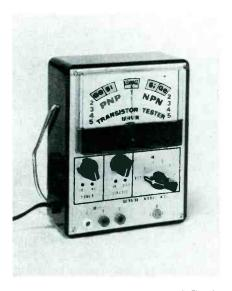
The unit operates on AC, is equipped with a wire-type handle which serves as a tilt stand for easier viewing, measures  $6\frac{3}{4}$ inches x 5<sup>1</sup>/<sub>4</sub> inches x 3 inches and weighs 3 pounds.
