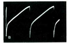
Fig. 5 Shorted turns in the winding of the vertical output transformer or an excessive resistance load across the transformer causes compression at the top of the raster. A) Typical compression at the top of the picture caused by an excessive resistance load across the vertical output transformer. B) Waveform at the yoke when there is compression at the top of the raster.
