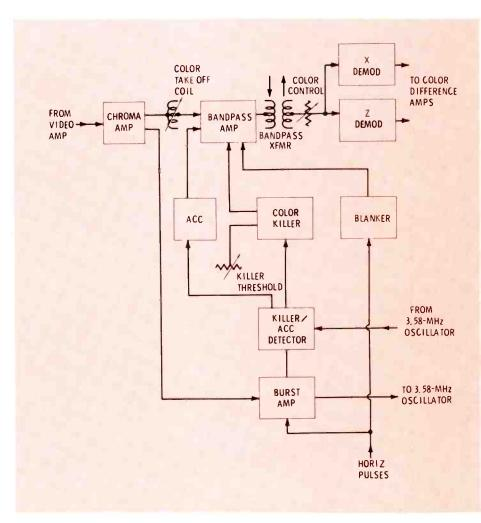
Fig. 1 This is the most common arrangement of stages in a chroma section. Some chassis might have a few more stages, like two bandpass amplifiers. The stage names might sound different: color IF, chroma amplifier, etc. But you'll find the relationships are remarkably the same regardless of who designed or who built the set.
