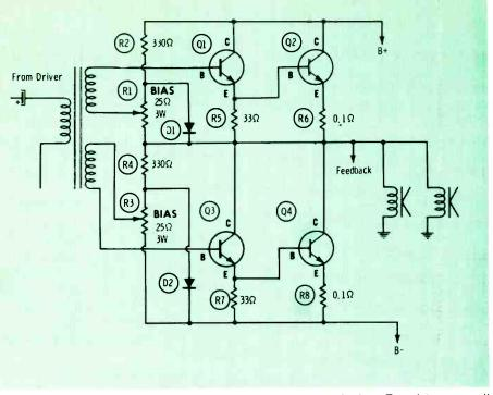
Fig. 4 Four-transistor design boosts output power even higher. Transistors are all NPN, but because they are driven by a special transformer they operate pushpull. The output is transformerless.
