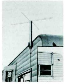
ble of receiving color and blackand-white TV signals on all UHF and VHF channels, as well as FM. The antenna can be folded down in seconds and enclosed in a weatherproof tube cap, ready for traveling, according to the manufacturer.
