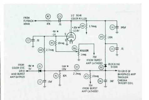
**Fig. 3** The automatic color control (ACC) line is short and simple. It includes D1, R1, C1, R2, R3 (which brings in a "bucking" voltage), and C6. The color-killer stage is isolated from the ACC line by diode D2 whenever a burst signal is present and the plate voltage of the tube is positive.
