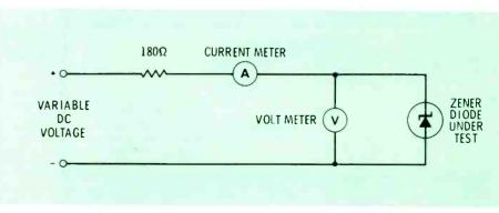
Fig. 1 Schematic of a circuit which can be used to test zener diodes by the voltagecurrent method.
