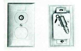
As the connector is withdrawn the house drop is terminated before the connection between the set and the drop is broken, preventing the generation of momentary standing-wave interference when the set is disconnected or moved to another outlet.
