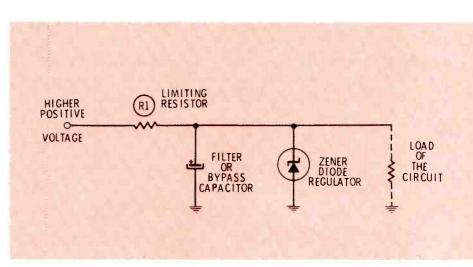
Fig. 5 Schematic of a typical power supply regulated by a zener diode. R1 limits the maximum current which can be drawn by the zener. The voltage across the load is regulated against input voltage changes or changes of the load current.
