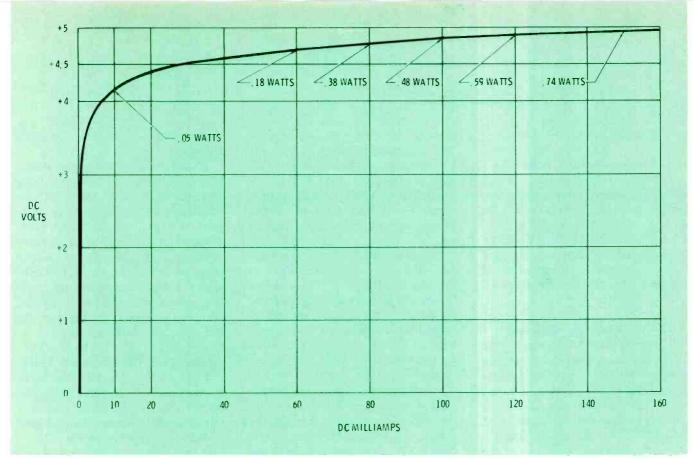
Fig. 2 Results of the voltage-current method of measuring zener diodes can be graphed. Shown here is the graph of an International Rectifier Z1102-C 1-watt zener diode. The nominal voltage rating is approximately in the center of the "plateau".
