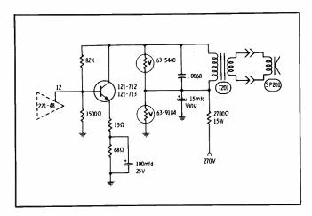
Do not service the receiver without a speaker or a load resistor connected across the speaker output leads, because the output transistor and the varistor can be damaged by the high peak voltages which can result.
