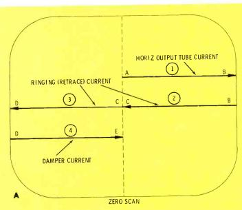
Fig. 1 Locations where the four steps of horizontal deflection occur on the screen of the picture tube, and also where they are located on the waveform of yoke current. This information can help technicians correlate visual symptoms with the area of the circuit where the defect is most likely to be. A) Power to scan from the center of the picture tube screen (point A) to the right edge (point B) is supplied by plate current of the horizontal-output tube. Current from
