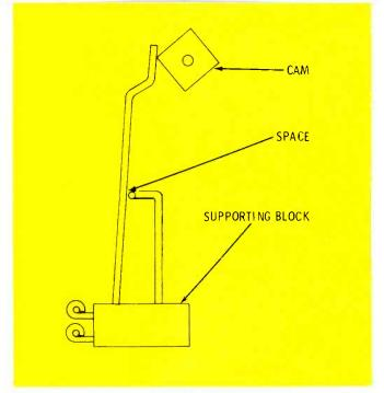
Fig. 9 Drawing of cam-type of cassette-stop sensor mechanism.
