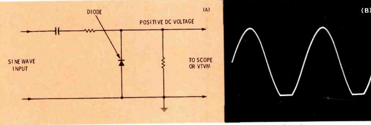
Fig. 5 Proof that a rectifier circuit in which the diode conducts during the negative-going peak of the waveform produces positive voltage. A) Circuit used for waveform and voltage measurements. B) Scope waveform showing that, because of the clipped negative peak, diode current during the negative peak produced positive DC voltage.
