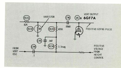
Fig. 8 Schematic of part of the vertical-output stage in the RCA CTC38A color TV chassis. The varistor "rectifies" the positive-going pulse from the plate of the output tube, producing a negative voltage, the amplitude of which varies with the amplitude of the pulse. This variable negative voltage changes the grid voltage of the output tube, to partially cancel any change in height.
