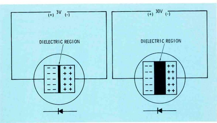
Fig. 1 Varactor diode with moderate reverse bias.
