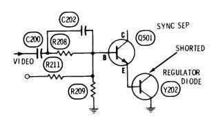
Symptom-no vertical or horizontal locking Cure-check diode Y202 and replace, if shorted
