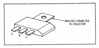
Replacement transistors, Zenith part number 964-27986, have an adequate heat sink that is part of the transistor and is connected internally to the collector. These extruded flat brackets, projecting from the tops of replacement transistors, should NOT be clipped to the aluminum shield, because this would short the collector circuit.
