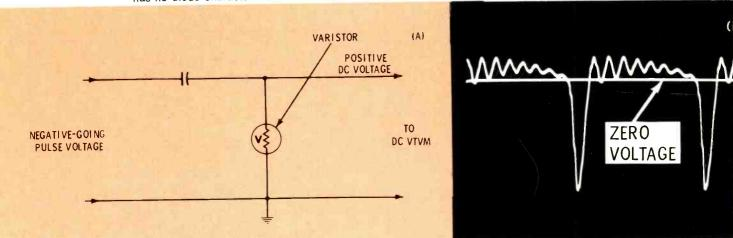
Fig. 7 DC voltage can be obtained from varistors, if the applied waveform is non-symmetrical. A) Circuit which produced the waveforms and DC voltages. B) Scope waveform of the input signal, showing the true zero voltage line. The negative-going voltage is greater than the positive-going.
