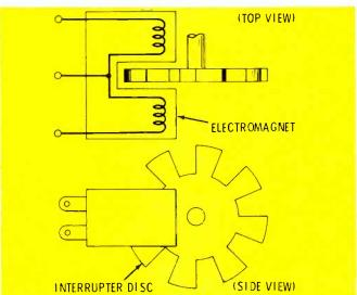
Fig. 10 Top- and side-view drawings of interrupter-disc-type of cassette-stop sensor.
