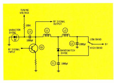
Fig. 3 Representative RF amplifier with bandswitching and varactor tuning.
