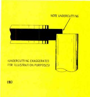
Fig. 13 A) Side-view drawing of take-up spindle drive mechanism. B) Enlarged view of drive shaft and rubber tire on take-up reel, showing undercutting of tire by shaft, caused by improper alignment and/or wear.
