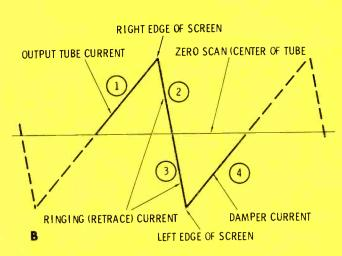
ringing of the yoke circuit moves the electron beam, in two separate steps, to the left side of the screen (point D). Current from damper rectification moves the beam from the left edge (point D) to the zero-current center of the picture tube screen (point E). These four steps constitute one cycle of horizontal scan. B) The same four steps of horizontal deflection as they relate to the waveform of yoke current.
