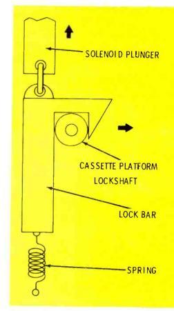
Fig. 12 Drawing of lock mechanism which holds cassette platform in play position until cassette-stop/eject amplifier energizes eject solenoid K1, Lock bar is then pulled up by solenoid plunger and cassette platform drops to "rest" position, forcing cassette out slot in front of player.
