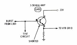
Symptom—missing or weak color Cure-check transistor Q401 and replace, if shorted
