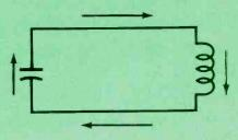
The capacitor voltage (source) was zero, and the "negative" coil current was maximum at point "C".
