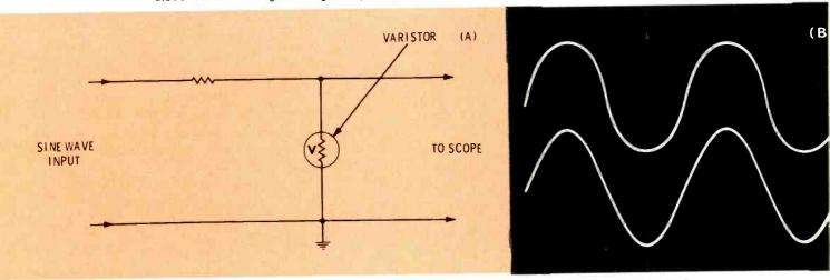
Fig. 6 A varistor passes the same amount of current whether the applied voltage is positive or negative, provided the amplitude of the applied voltage is the same. A) Circuit of a sine wave applied to a varistor. B) Bottom waveform is the input sine wave for comparison; both the positive and negative peaks of the top waveform have been rounded by varistor current. The existence of identical positive and negative alterations prove that a varistor has no diode characteristics.
