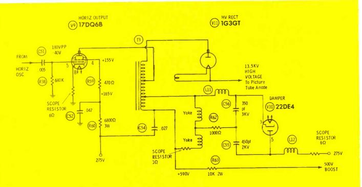
Fig. 5 Complete schematic of the horizontal sweep and high-voltage section of the Sears 456/528.51912 b-w television chassis. Normal DC voltages for this one individual chassis are included. Waveforms will be added next month, to illustrate a detailed discussion about troubleshooting the horizontal sweep sections of television receivers.
