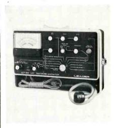
Other features include: continuously adjustable element voltages, for "as needed settings"; automatic rejuvenator rate control; RC timer; 0 to 40-volt heater potentials available; 117 VAC, 60-Hz operation; 41/2-inch scaled meter.
