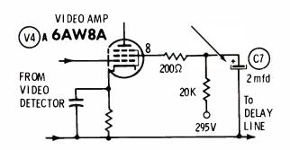
Symptom—smeared picture and poor vertical locking Cure-test C7 by replacement; the value is not critical
