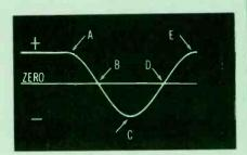
Shows the power supply voltage and the first cycle of the sine wave of coil current. Beginning and ending points of each 1/4 cycle are indicated by letters.
