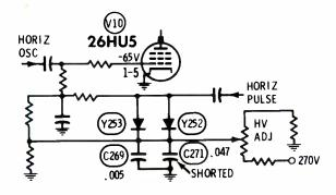
Symptom—dim raster; reduced high voltage Cure-check C271 and replace, if shorted
