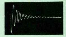
A DC supply voltage was connected to a tuned circuit long enough for the current to reach maximum. When the power supply was suddenly disconnected the damped wavetrain of sine waves shown here was produced. The first 1/4 cycle is not displayed on the scope screen because the vertical amplifier section of this particular triggered-sweep scope is not equipped with a delay line.
