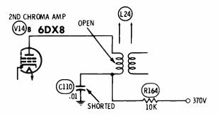
Symptom—no color; no plate voltage on pin 6 of V14 Cure-check for open transformer L24 or shorted C110 and burned R164
