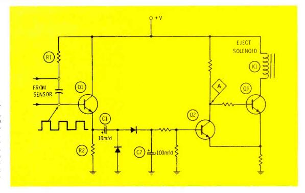
Fig. 11 Typical cassette-stop / eject amplifier, which controls current to the eject solenoid, K1. Input to the amplifier section is the pulses from the sensor mechanism. See text for details of operation.
