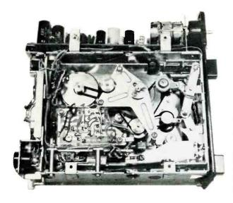
Fig. 4 Bottom view of Automatic Radio Model ACS-6000 casette tape player, which used a belt-drive system between motor and flywheel and take-up sprocket,
