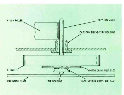
Fig. 6 Side-view drawing of capstan and flywheel assembly used in most automotive cassette tape players.
