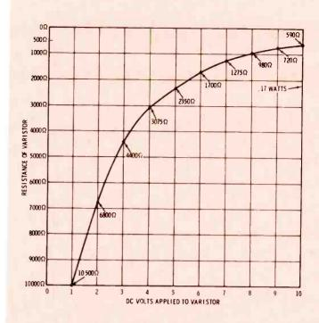
Fig. 3 A graph of applied voltage versus resistance can be computed by Ohm's law, using the values in Fig. 2.
