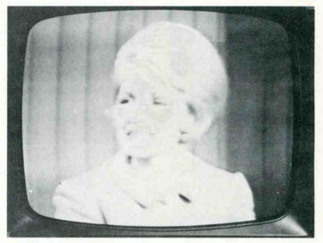
**Fig. 3** Slow warmup and "sparkly" overload at high brightness and contrast characterize CRT with weak emission or gas. Focus may get bad as symptoms progress, but the main sympton usually annoys the viewer first.
