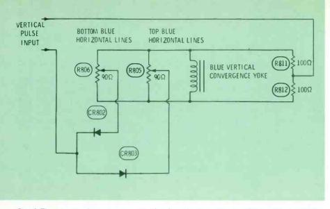
**Fig. 6** The blue vertical convergence circuit varies both the amplitude and phase of the voltages applied to the blue vertical coil in the RCA CTC54 color TV chassis. The two diodes clip the deflection waveform into pulse and sawtooth, for correction of tilt and amplitude.
