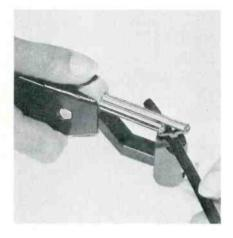
Any type of cable insulation may be stripped, including **Teflon**, **KAP**-**TON**, **KEL-F**, and a complete range of low-temperature cable coverings, according to the manufacturer.
