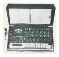
The "Programmed Section" has 9 sockets for testing other tubes by operation of lever-action switches for each pin. A lever reportedly is provided to simultaneously clear the setting of all the switches.
