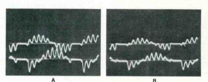
Fig. 6 Outputs of B-Y and R-Y amplifiers (bottom and top respectively). (A) Normal waveform (B) Nulls shifted to right.
