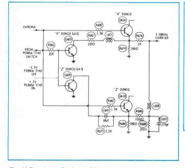
**Fig. 14** Transistors Q603 and Q605, shown here, are used as switches in the Sylvania E01 color chassis, to add L603 and C643 to the circuit which determines the phase difference between the two demodulators.
