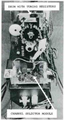
**Fig. 24** This rear view of the tuner assembly shows the box containing the precision tuning resistors, and the channel-selector module.
