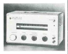
A slide-rule type dial with mirrored-scale is provided to minimize parallax reading errors.
