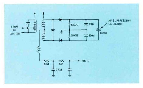
Fig. 3 Some FM receivers employ other noise-suppressing circuitry in addition to the limiter stage. For example, the ratio detector circuit shown here is equipped with a 10-mfd capacitor, to suppress, or filter out, noise impressed on the signal by amplitude modulation.
