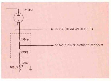
Fig. 5 Less-common focus system is supplied voltage from bleeder and divider across picture-tube high-voltage stage. Has same advantage as multiplier version: changes whenever high voltage changes.
