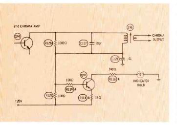
Fig. 2 Illumination of the Philcomatic Lite indicates that the color killer is inactivated and color should be received. When the 2nd chroma amplifier transistor conducts, the voltage dropped across supply resistor R129 forward biases Q97 into conducting, and the collector current lights the indicator bulb.
