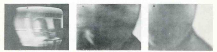
Fig. 1 Proper analysis of focus requires close-up examination of the raster. The blurred picture in (A) is actually caused by video smear, not by poor focus; you can tell the difference if you examine closely the raster lines, as in (B), which shows how the
