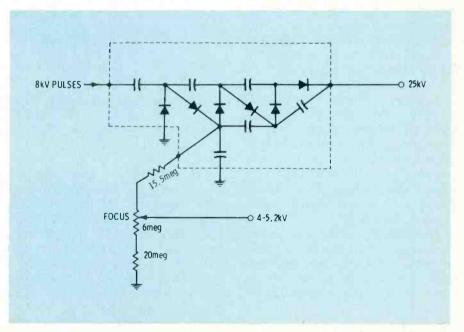
Fig. 4 High-voltage multiplier is the trend in color sets. It makes focus voltage easily accessible from a tap on the multiplier. Resistive divider steps down DC voltage to that needed by color CRT focus element.
