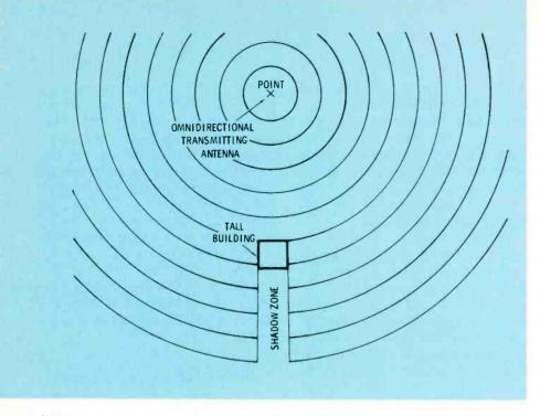
**Fig. 7** The inability of the relatively short FM waves to bend around obstacles causes "shadow zones" in the propagation pattern of an FM transmitting antenna. Such zones of weak or missing signals are common in urban areas.
