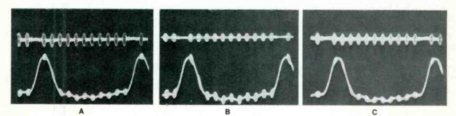
Fig. 4 Output of 2nd chroma amplifier (top) and input to burst amplifier (bottom). (A) Normal waveform (B) Gate pulse leads burst (C) Burst leads gate pulse.
