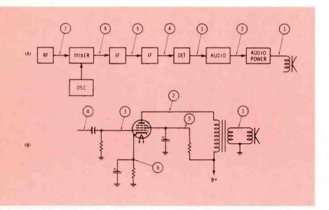
Fig. 4 Signal injection sequence. Follow it stage by stage. Trouble lies between the point where signal gets to speaker okay and the point where the symptom is reproduced.
