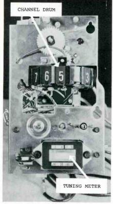
Fig. 23 The front of the varactor tuning assembly has a conventional-appearing drum. However, the drum is not connected to the tuner. The tuning meter reads the tuning voltage, to estimate the channel in use during the setup procedure.
