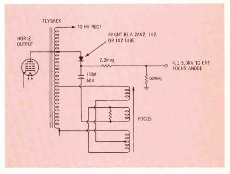
**Fig. 6** Inductive focus control in this circuit is a transformer which applies an out-ofphase pulse at the opposite side of the focus rectifier. Moving the inductance core varies how much DC is applied to CRT focus anode.
