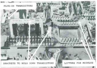
**Fig. 22** The larger transistors on the Zenith 25CC55 color chassis are held in their sockets by plastic hold-down brackets. Plastic strips are installed under the terminals at each end of the modules. Lifting up on the plastic strips safely removes the modules.
