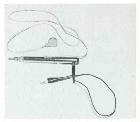
**Fig. 6** Chip transistorization and integrated-circuit technology make signal tracers like this possible. The instrument in Fig. 1 also functions as a tracer, with AF and RF positions selected by a switch on the handle.
