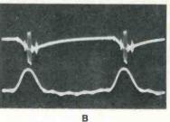
Fig. 5 Output of burst amplifier (top) and input to burst amplifier (bottom). (A) Normal waveform (B) Chroma leaking through amplifier distorts burst.
