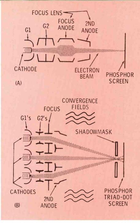
**Fig. 2** Electron gun in monochrome picture tube (A) includes focus "lens" that, in modern CRT's, assures good focus over very wide range of focus-anode voltages, sometimes even at ground potential. Color CRT is shown in (B).
