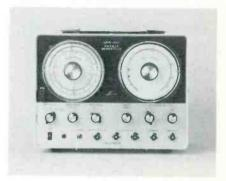
A marker oscillator, said to be of the post-injection type, is employed, and a control is provided to vary the amplitude of the marker. The marker oscillator is continuously variable in 4 bands, and reportedly has provision for crystalaccuracy calibration by means of a crystal socket mounted on the front panel.
