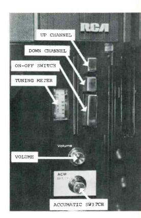
Fig 11 View of the top part of the frontpanel controls on the RCA CTC54 chassis.
