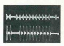
Fig. 2 Output waveforms of video detector (bottom) and 2nd chroma-bandpass amplifier (top). (A) Normal waveform (B) Result of tuning toward sound.
