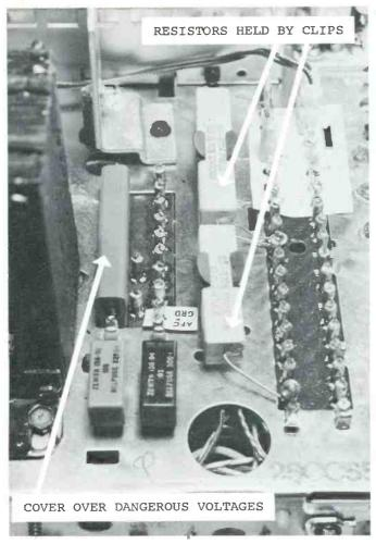
**Fig. 20** Large resistors held by spring clips and an insulating cover over terminals having dangerous voltages are two safety and serviceability features of the Zenith 25CC55 color chassis.
