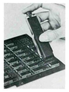
To extract an IC, the tool reportedly is positioned over the component to be removed and the stainless steel spring removal clip is lowered until the clip jaws are under the IC base. Squeezing the clip securely grips the component. Lifting the tool pulls the IC free; pressing the top button ejects it from the tool.
