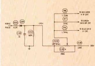
**Fig. 3** Different ratios of DC coupling between the -Y amplifiers and the grids of the CRT are provided by this circuit in Philco 22ST80/81 and 21ST91P color TV chassis. Better reproduction of complementary colors is the primary function of this circuit.
