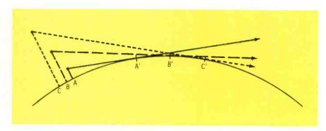
Fig. 5 How increasing the height of the transmitting (or receiving, or both) antenna increases the "line of sight" of the radio.
