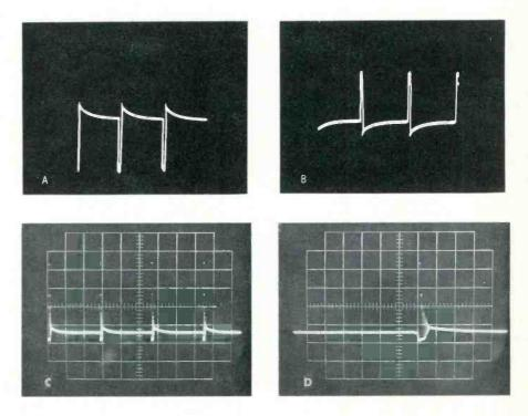
Fig. 2 Signal-injector outputs tend generally to pulse waveshapes. (A) shows a sharpsided pulse on a service scope, and (B) is the same signal if the battery and transistor were the other polarity. Waveform (C) was taken on a triggered scope because it is a series of little bursts of oscillation and isn't easy to see on a regular scope. (D) is one pulse, considerably magnified by the triggered scope.
