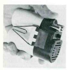
used by itself to generate a 400-Hz tone when continuity exists between the terminals under test.
