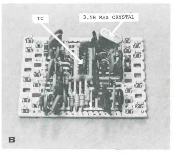
Fig. 19 Two of the Duramodules used in the Zenith 25CC55 color chassis. (A) One IC is used on the video and AGC module. (B) One plug-in IC is the only solid-state device used on the 3.58-MHz carrier module.
