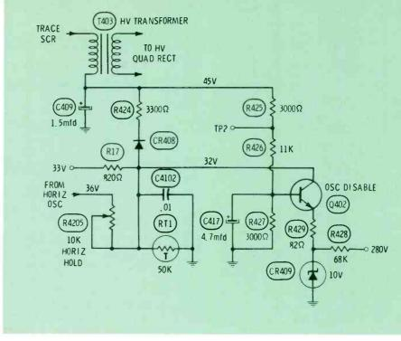
**Fig. 8** In the event of excessive high voltage in the RCA CTC54 chassis, the oscillator disable circuit forces the horizontal oscillator far off frequency. This is accomplished by Q402, which, when the high voltags is too high, conducts and reduces the 32 volts at one end of the horizontal-hold control to about 10 volts. See text for a more detailed explanation of the circuit operation.
