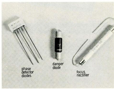
**Fig. 1** Examples of "high-voltage" rectifier assemblies and a phase detector duo-diode.
