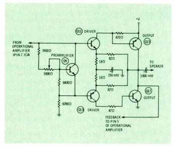
Fig. 9 Preamplifier/driver/audio-output circuitry used in Bendix 1972 radio design is relatively new to auto radio.
