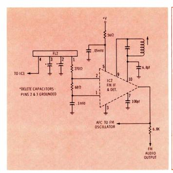
Fig. 4 IC shown here, used in Bendix's new stereo FM auto radio, performs the functions of amplifier, limiter and quadrature detector.
