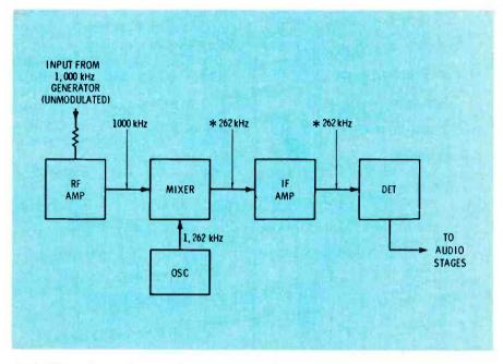
Fig. 8 "Signal tracing" in a radio by measuring the frequencies of the signals at key test points, as shown here, is an example of how a DFC can be applied to conventional troubleshooting techniques. Frequencies shown here are for an auto radio.
