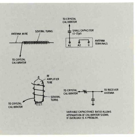
Fig. 4 Shown here are several methods for connecting the crystal calibrator to a receiver.
