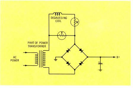
Fig. 1 Typical automatic-degaussing circuit.
