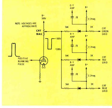
Fig. 2 CRT grid clamping circuit, typical of that employed in 1967-71 RCA color TV chassis.
