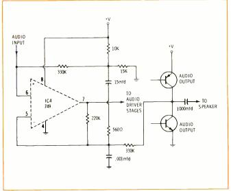
Fig. 8 IC operational amplifier functions as a predriver audio amplifier in new Bendix radio. See text for details.
