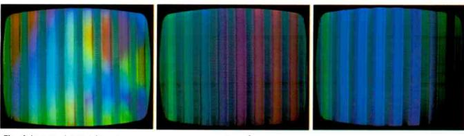
Fig. 4 Impure picture tube can cause wrong tints and weak color. Color bars become a patchwork of hues when the purity is poor. The bars near the center are nearly white (no color).
