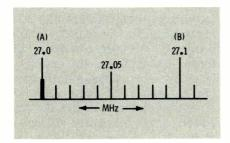
**Fig. 5** Calibrated dial of a hypothetical receiver calibrated for a portion of the 27-MHz Citizens' Band.
