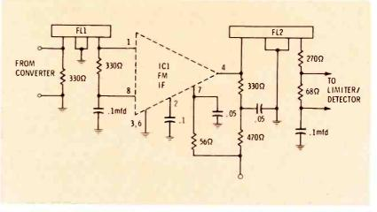
Fig. 3 Ceramic filters provide input and output coupling in IC-equipped FM IF amplifier section of Bendix's 1972 auto radio.
