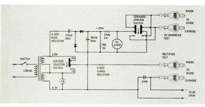
Fig. 6 Schematic of a test jig you can build to test high-voltage rectifiers by both the high-voltage ohmmeter and rectified-voltage methods.
