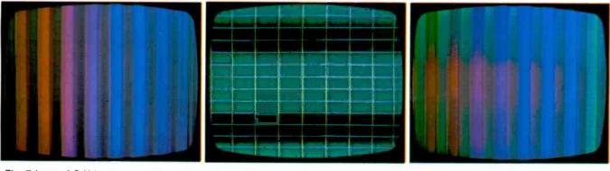
Fig. 7 Loss of G-Y is not very noticeable either on the bars, as shown here, or during colorcasts. A weak green is created by the -Y action of the other two demodulators, which remove red and blue from the raster so that some green remains.
