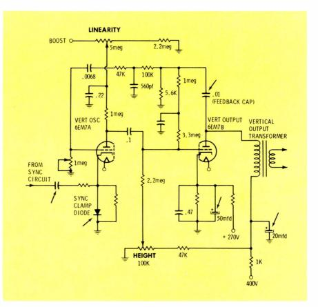
Fig. 4 Arrows point to areas which might cause vertical sync instability without a related sweep defect.
