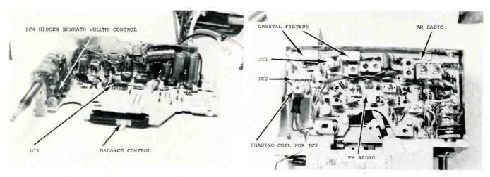
**Circuitry** of Bendix's new AM/FM Stereo FM auto radio is contained on two subassemblies: (Left) Multiplex/audio/power supply subassembly. (Right) AM and FM RF and IF subassembly.
