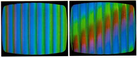
**Fig. 12** Smeared colors are the result of misalignment; to produce the example shown here, the fine tuning was misadjusted. Note that the color saturation was not reduced noticeably because of ACC action. Always adjust the fine tuning to produce sound bars and beat patterns, then reverse the rotation only enough to eliminate the beat patterns.
