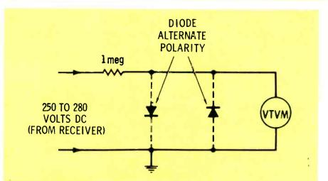
Fig. 2 Schematic diagram of a setup for testing "high-voltage" rectifiers by the high-voltage-ohmmeter method.
