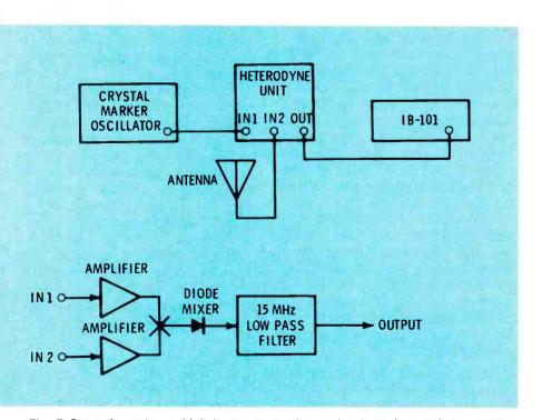
Fig. 7 Setup for using a high-frequency marker and a hetrodyne unit to measure frequencies above the range of the IB-101.
