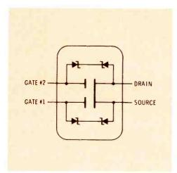
Fig. 2 Built-in Zener diodes protect new MOSFET's from static charges which frequently destroyed previous designs of MOSFET's.
