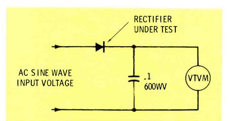
Fig. 3 Schematic diagram of setup for testing rectifiers by the rectified-voltage method. The input voltage should be selected to match the rating of the rectifier. Leakage through the rectifier reduces the output voltage. The higher the output voltage, the better the rectifier.
