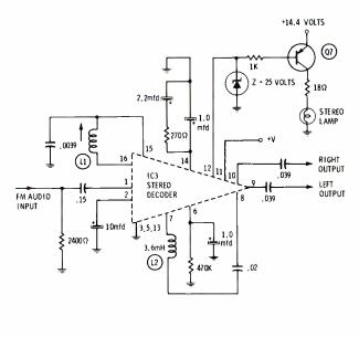
Fig. 5 IC-equipped stereo decoder circuitry of new Bendix radio is simpler than previous IC designs. Note that only one adjustment is required -L1.
