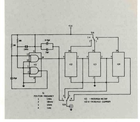
Fig. 3 Circuitry of an extremely accurate crystal calibrator. Application of the calibrator is explained in detail in the text.
