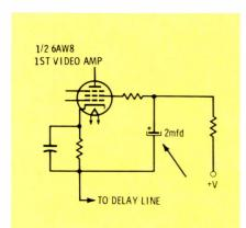
**Fig. 3** Vertical locking problems can be the result of defective electrolytics in video amplifiers.
