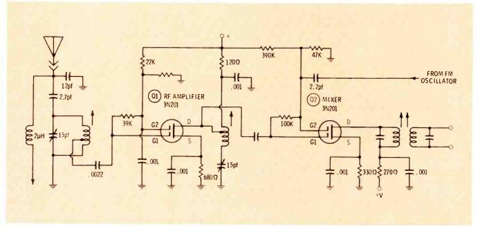
Fig. 1 Schematic diagram of the "front end" of Bendix's new stereo FM auto radio. Note the use of dual-gate MOSFET's.
