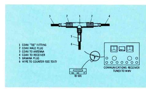
**Fig. 2** Equipment connections for calibrating the time-base oscillator of the IB-101 by zero beating its output against a signal from WWV. The receiver used should be equipped with an S-meter. See text for procedure.
