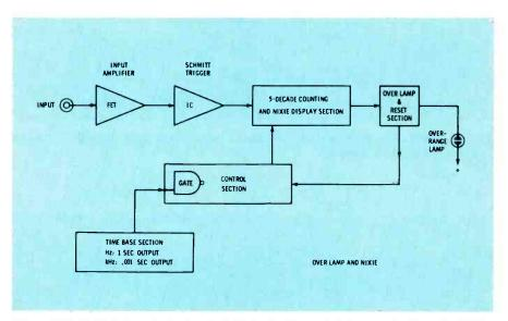
Fig. 1 Simplified block diagram of Heath's IB-101 digital-frequency counter (DFC).
