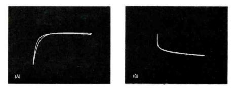
Fig. 5 Most of the high-voltage rectifiers tested were not supplied enough voltage by the Eico 443 curve tracer to produce meaningful curves. A) Peak-inverse-voltage curve of the boosted-boost rectifier appears similar to that of power-supply diodes, except the avalanche point (on the left) does not have a sharp corner. B) Nearly 6 volts of forward voltage drop was measured during this test of the damper diode. A power-supply diode measures about .7 volt.
