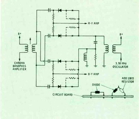
Fig. 3 Dotted lines show how resistors are added to prevent diode radiation.
