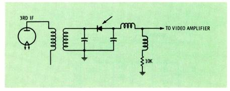
Fig. 5 A defective diode can cause sync and/or AGC defects.
