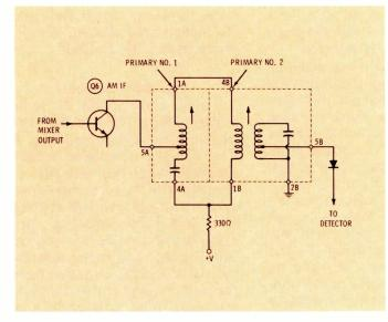
Fig. 7 Circuit diagram of new "dual-can" AM IF amplifier transformer and associated circuitry used in Bendix 1972 radio design.
