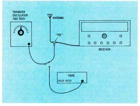
Fig. 6 Equipment connections for using the transfer-oscillator method of measuring frequencies above the range of the IB-101.
