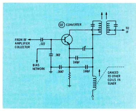
Fig. 9 Circuit diagram of a typical converter stage in an auto radio.
