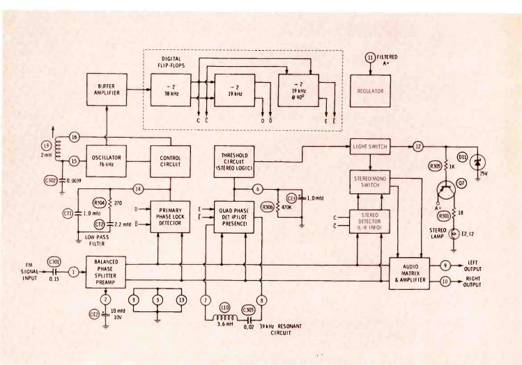
Fig. 6 Block diagram of the internal circuitry of the stereo decoder IC used in Bendix's new auto radio. See text for detailed explanation.
