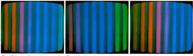
**Fig. 1** Color bars displayed by a normally operating receiver which has 105-degree separation between R-Y and B-Y. Slightly excessive width has obscured the 10th bar and shows only a part of the 2nd bar. The brightest red bar is the 3rd from the left.
