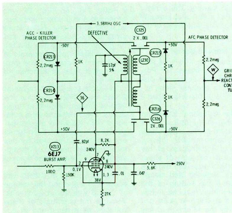
**Fig. 12** Schematic of the burst separator stage in Zenith 14B9C50 color chassis shows many components which could cause loss of color locking and, in turn, loss of color because of killer action.
