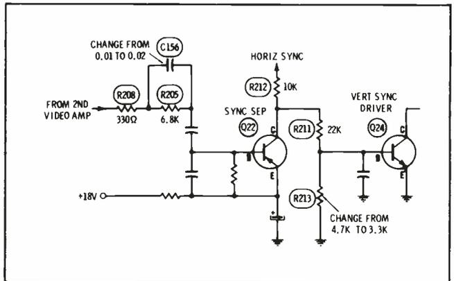
of C156 from .01 to .02mfd, and changing the value of R213 from 4.7K ohms to 3.3K ohms, as shown here.
