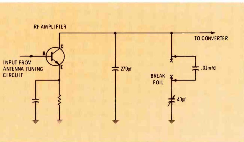
**Fig. 9** In humid areas there is a high incidence of trimmer capacitor faults. To troubleshoot, break the foil to the trimmer and series connect a .01M-fd capacitor. If the noise stops, replace the trimmer.
