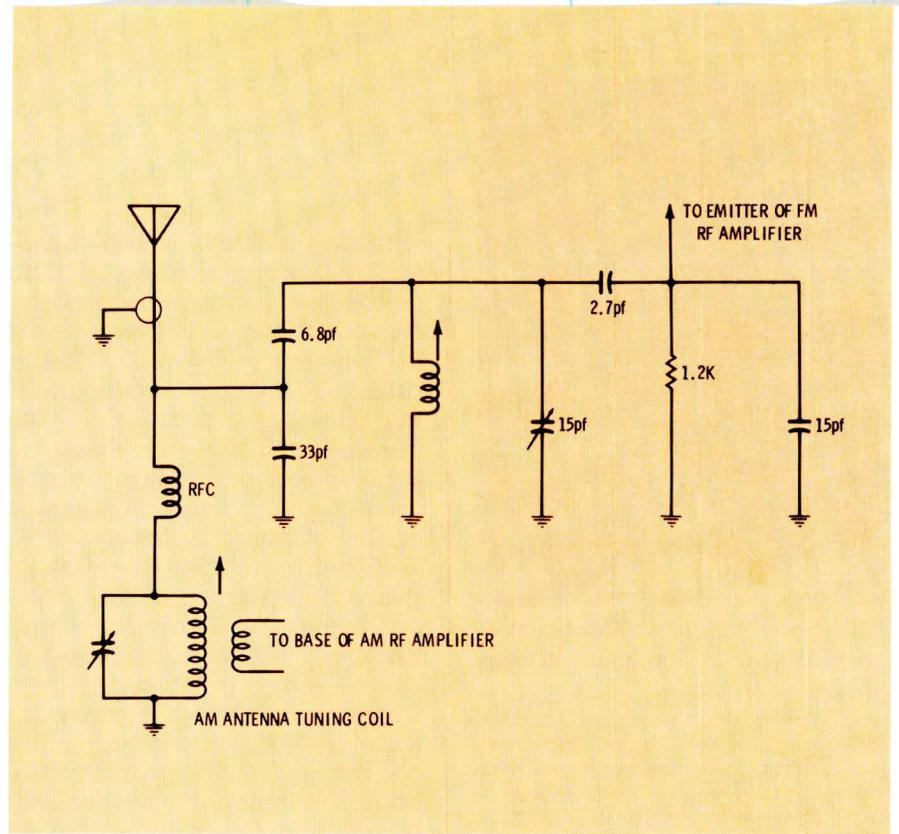
**Fig. 10** The antenna of FM auto radios usually is electrically connected across a capacitive voltage divider, so that the antenna is matched to a higher "Q" and more selective tank circuit. Some models, a minority, use a one- or two-turn link around the "cold" end of the RF input coil, to match the antenna through transformer action.
