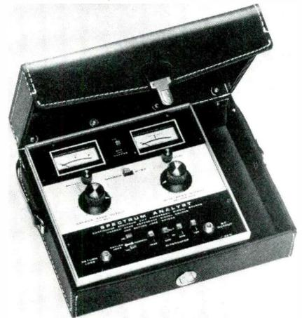
impedance is 75 ohms with a VSWR of 1.1. **Return loss bridge—**impedance is 75 ohms, balance is 40 dB minimum, the unterminated output reference level is 1 millivolt, and the flatness of response is  $\pm 2$  dB, or better. **Operating temperature—**+30 degrees Fahrenheit to +100 degrees Fahrenheit. **Battery—**continuous usage before recharging is 6 hours for wide-band operation or 36 hours on narrow-band
