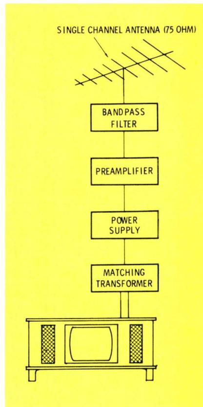
**Fig. 1** A simple single-channel antenna system for reception of distant TV signals.
