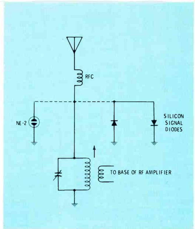
**Fig. 6** Static discharges through the antenna circuit can destroy the RF transistor. Diodes or neon discharge lamps are often used to drain the charge before it "hits" the transistor.
