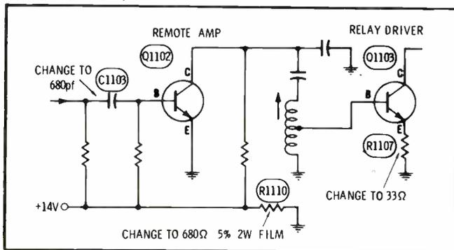
1) Check the values of R1107 (33 ohms) and R1110 (680 ohms, 5 per cent, 2-watt, film); replace these resistors, if the values are not as listed here.
