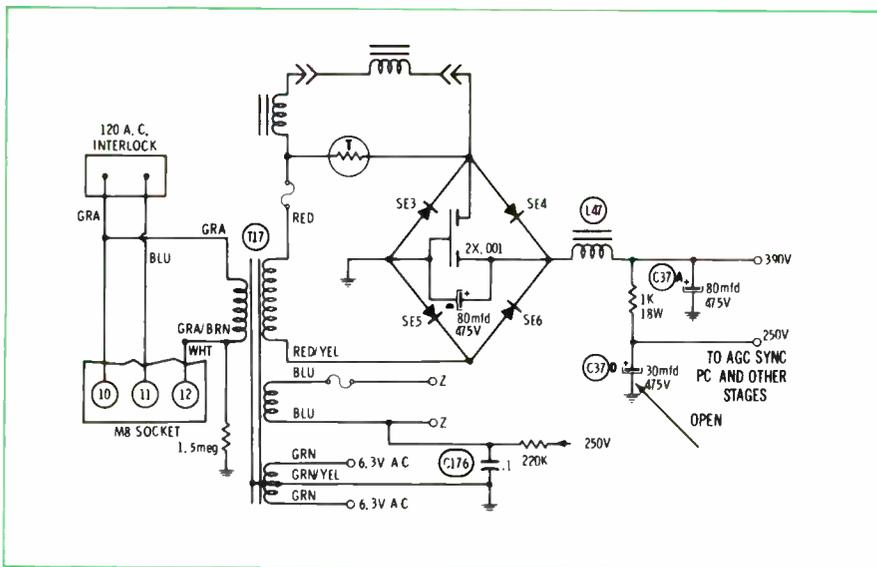
Fig. 7 Schematic of the power supply in Zenith 20X1C38 chassis.
