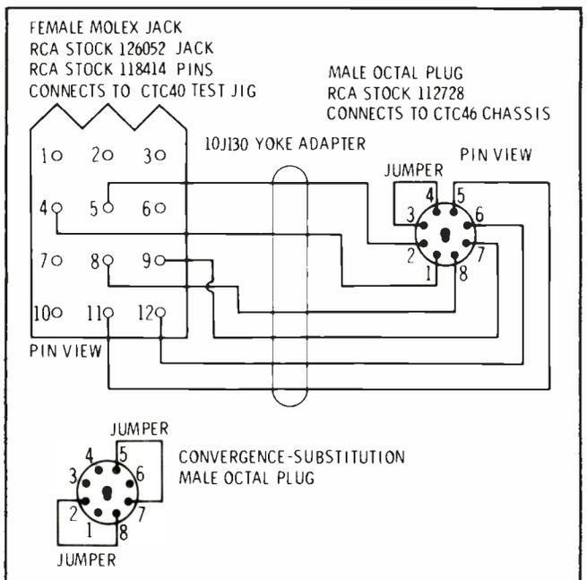
Convergence components of the test jig should not be used with the CTC46 chassis. A male octal plug equipped with two jumper wires, as shown here, should be used as a substitute for the convergence assembly.
