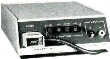
supplied by an internal battery, but there are options for rechargeable batteries or for line voltage operation. The multimeter turns on by a push-to-read switch on the probe, and a stable reading is obtained in less than 2 seconds. Typical battery life for push-to-read operation is about 3 months. Overload protection is provided. For example, full line voltage can be applied, without damage to the multimeter, across the input on the ohmmeter function.
