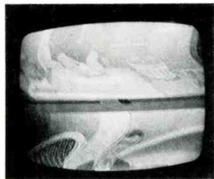
Fig. 6 The screen of the Zenith 20X1C38 color chassis displayed an "S" curve and instability of the AGC and vertical locking when C37D was open.
