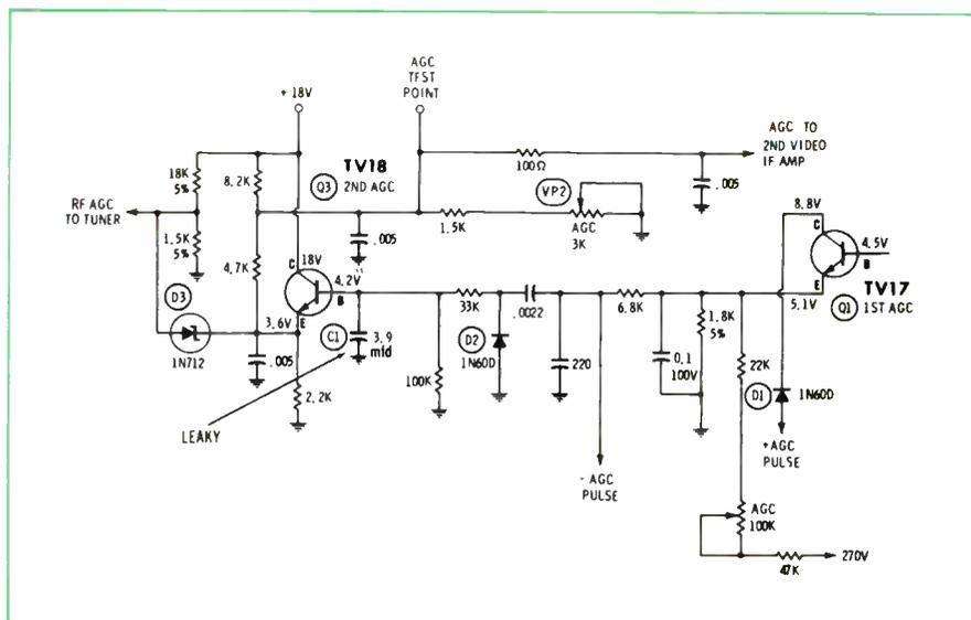
Fig. 9 Schematic of the transistorized AGC circuit in Philco 19QT87/B color chassis. Several components which can cause AGC overload are listed in the text.
