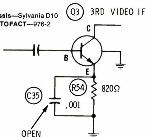
**Symptom**—Insufficient sensitivity; no snow off channel
