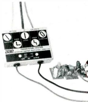
scope, the unit tests diodes, and the junctions of bi-polar transistors. Resistors show as a slanted line, and capacitors produce a circle. Tests in-circuit diode and transistor junctions, resistors and capacitors. Typical patterns are printed on the panel of the instrument.
