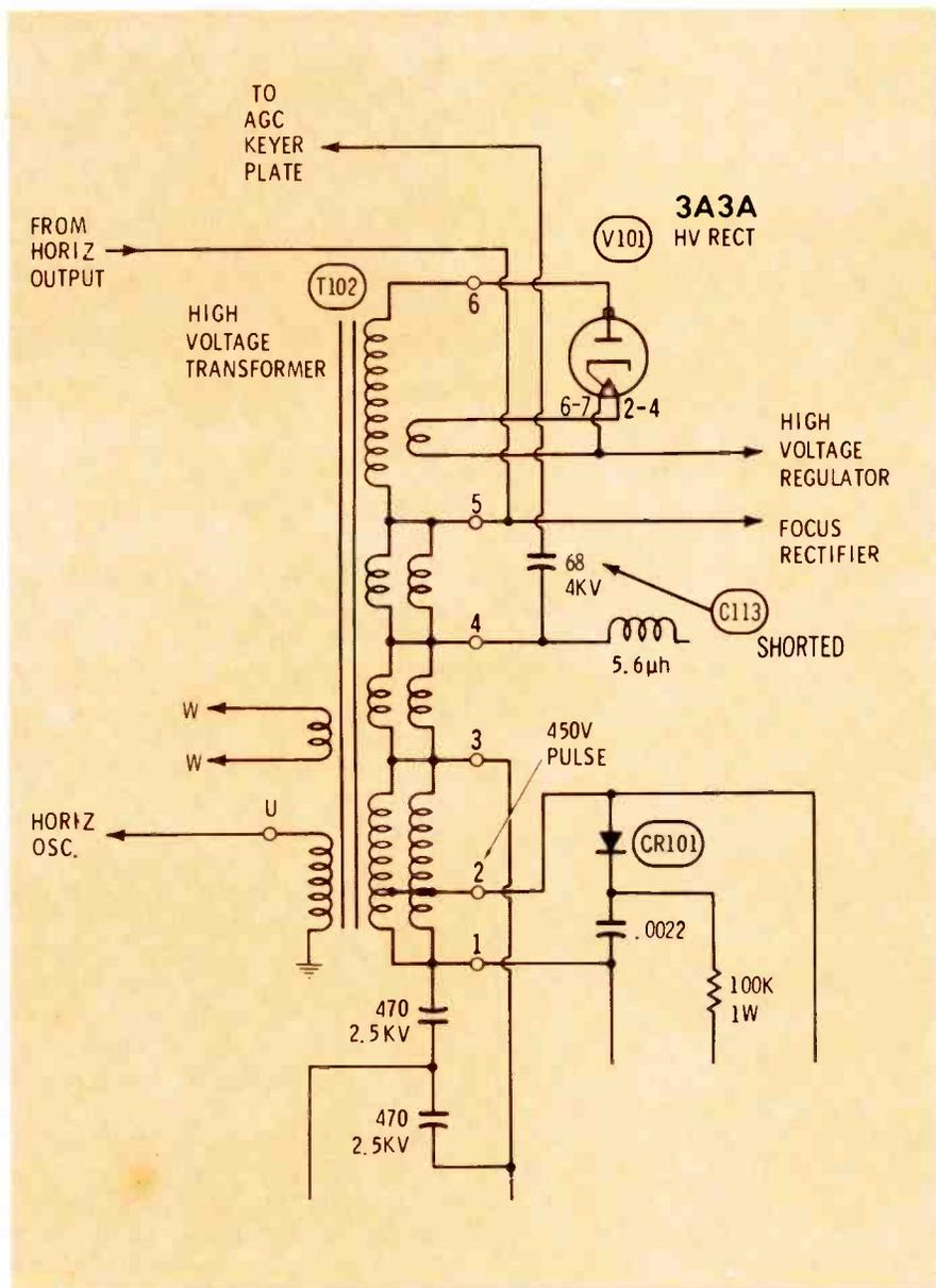
Fig. 5 Partial schematic of the horizontal-sweep circuit in RCA CTC25X color chassis. Capacitors eliminated the high voltage.
