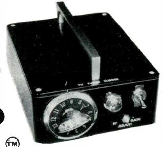
Transistorized Test Unit substitutes the tuner in defective TV Receiver to prove whether original tuner is good or bad.
