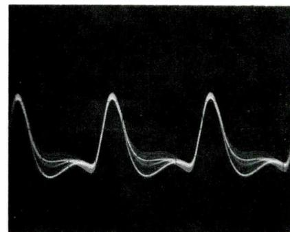
Fig. 8 This large 16-volt p-p waveform was produced at the 250-volt supply when C37D was open.
