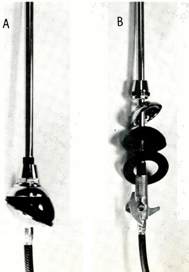
of these antennas require two holes in the fender. The difference is that the DSSC requires two large holes while the SSSC requires one large and one small hole. The DSSC stanchions can be adjusted for any spacing relative to the mast length and each other.
