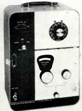
**Features:** Continuous frequency coverage up to 470M-Hz, electronic fine tuning, low RF leakage, automatically-controlled output voltage, and optional internal or external amplitude modulation.
