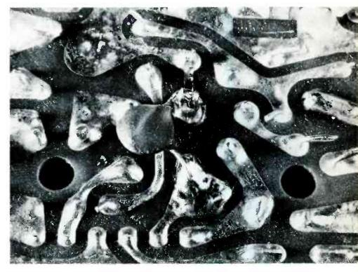
Fig. 2 Wire the added capacitor point-to-point, and shorten the length of the leads as shown.
