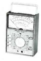
from 1 ohm to 100 megohms, conventional or low voltage modes; decibel ranges from -40 dB to +62 dB; and DC null scale with 1 mV resolution.
