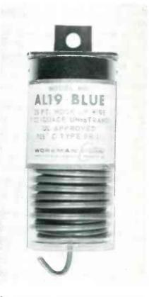
Specifications: The hook-up wire container is 1 3/8 inches x 3 inches. The wire is 7/22 (22 gauge unistrand) UL approved, can withstand temperatures to 105 degrees centigrade, type FR-1. Price: Not available
