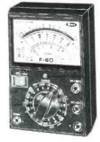
**Features:** A zener diode provides meter protection, a Span-Band type of pivot is used for low friction of the pivot bearings, silverplated switch contacts and a mirrored scale are provided.
