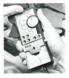
the wires. A "stop-lock" feature holds the reading for as long as required for measurements made in the dark or in positions where the meter could not be seen at the time. By use of test leads, AC voltages up to 600 volts can be measured, and resistances from 1 ohm to 1,000 ohms. A simulated-leather case with a compartment for storage of the test leads is provided.
