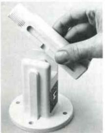
upper section is folded in one direction, the antenna is horizontal; folded in the opposite direction, it slides free of the deck mounting assembly for storage. Specifications: The mount is furnished with three tapered spacer discs to permit vertical positioning of the antenna on surfaces sloping as much as 6 degrees.
