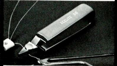
This is No. 80, Xcelite's little gem for absorbing and dissipating heat when soldering fine wires or working close to delicate electronic components. Solder won't adhere to copper jaws because they're nickel plated. They're spring loaded to "stay put" and have a smooth surface to avoid marring or scratching.
