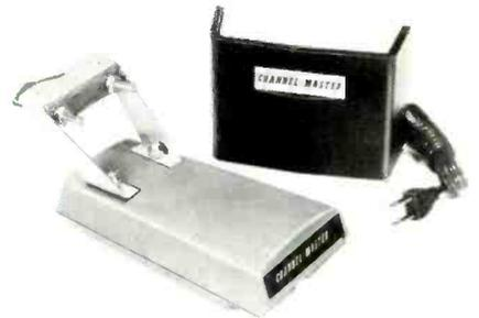
Specifications: Full gain is typically 45 dB for all TV channels and FM, when the low-band and high-band gain controls are fully open. Seven channel output capability is 59 dBmV (0.9 volts) for each low-band channel and 54 dBmV (0.5 volts) for each high-band channel. Input and output impedances are 75 ohms, and the noise
