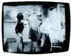
Fig. 5 When C248 was removed for a test, the picture was small on all four sides of the raster.
