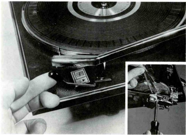
**Step 15** Where cueing is a part of an automatic turntable, damping often is provided to keep the tone arm from dropping abruptly and damaging the stylus tip or the record. Below, the cue handle. At right, adjusting limit of cue lift, so arm doesn't go too high.
