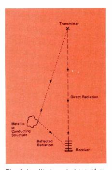
**Fig. 1** Amplitude and phase of reflected signals can change a signal-strength reading 3 dB's or more.
