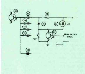
Fig. 6 Voltage switching of a diode for each crystal allows simple circuits to scan eight channels.
