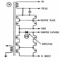
Symptom—Picture 3 inches to the right Cure—Replace defective X20 centering diode
