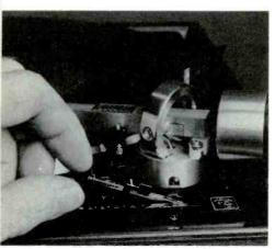
**Step 8** Sideways movement of tone arm across record grooves towards the center is called skating. To minimize this unwanted effect, designers include some means of countering it. The feature goes by the name antiskate. This one, consisting of a bar connected by a cord to the tone arm, has a sliding weight that determines how much anti-skate pressure is applied.
