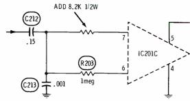
Symptom—Failure of audio IC because of arcs Cure—Make sure C134 is grounded to shield braid, replace IC and add a 8.2K resistor in series with pin 7, as shown
