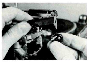
**Step 2** Many costly changers, and most hi-fi turntables, have knob for setting exact stylus pressure. This one, not the most expensive, uses spring tension to counterbalance weight of arm and cartridge.
