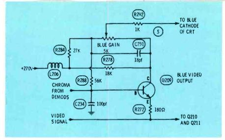
Fig. 8 Schematic of the b-w and color matrixing in a blue video amplifier stage.
