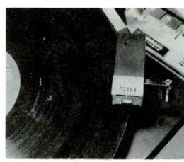
**Step 10** This is the vertical tracking adjustment on a high-quality turntable. You saw a cartridge in Session 1 that needed this adjustment corrected. It looked sideways in its mounting, viewed from the front. The stylus can't seat properly in the groove unless this is right.
