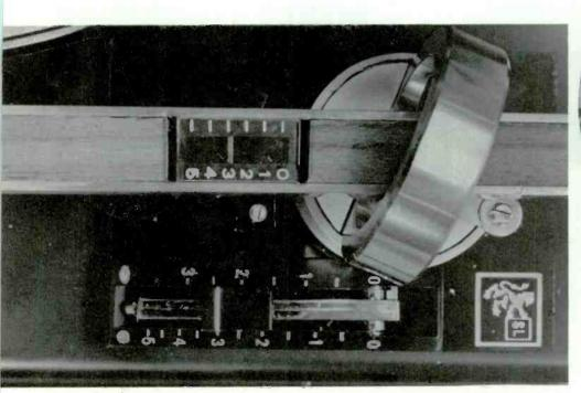
**Step 6** After the tone arm is balanced, the grams scale is accurate. You dial in the stylus pressure recommended for the cartridge being used. If the cartridge is changed, the tone arm must be rebalanced at zero, and the new stylus pressure then set on the dial.
