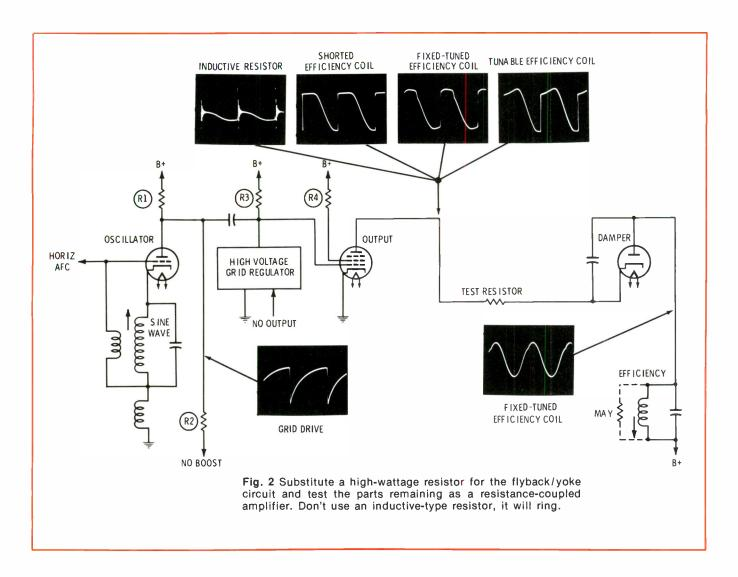
the damper cathode and the output plate. This changes the circuit of Figure 1 into the simple circuit of Figure 2. Presto, the horizontal-output stage has been transformed from a very complex stage to a fairly simple resistance-loaded amplifier. If it performs properly, the fault must be in the flyback-yoke circuitry. If it doesn't do its job, the tests described below will pinpoint the trouble.
