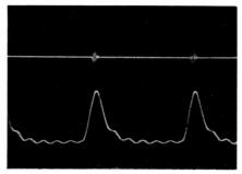
Fig. 4 Examples of wrong phase of the keying pulses. (Left) Top waveform is the colorcast chroma at the input to the keyer. Bottom waveform is the keying pulse, incorrectly delayed too much. (Right) Top waveform shows the weak burst at the plate caused by the wrong phase of keying pulse.
