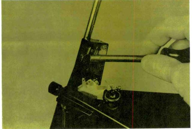
**Step 12** How high the tone arm lifts is determined by a screw underneath the tone arm, on this record changer. Might take a nutdriver, a Phillips, or regular screwdriver.
