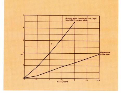
Fig. 2 The effects of VSWR and transmission line length on signal strength.
