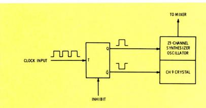
Fig. 1 Block diagram of a two-channel CB scanner circuit. A digital J-K flip-flop alternately grounds the synthesizer then the channel-9 crystal to permit monitoring of two channels.
