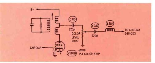
Fig. 13 Schematic of a chroma stage in which an intermittent was located.
