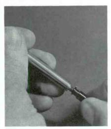
Step 18 In one automatic turntable, the pushoff adjustment is part of the spindle. A fork is part of the cycling mechanism. At the right time, the fork pulls downward on the bottom of this spindle, pulling rods inside it and dropping the record. The same pulling action causes the spindle to sense whether to shut off after the record plays.
