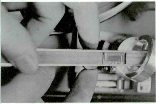
**Step 4** To begin adjustment, you first set the grams-scale knob to zero. This calibrates the knob to deliver exactly the indicated grams of weight at the stylus tip, but only after the arm is balanced.
