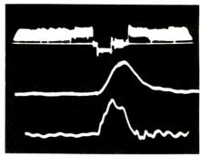
Fig. 2 Phase relationships of burst and keying pulses. Top waveform is the station video at the detector showing the burst to the right of the sync pulse. Bottom waveform is the raw horizontal pulse, whose tip arrives before the burst, making it unsuitable for keying. Center waveform has been delayed by R249 and C168 acting as a low-pass filter. The tip arrives at the same time as the burst.
