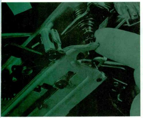
**Step 17** Dropping the record is a function of the spindle. But down underneath, something does the pushing. Here, it's a projection on the cycling slide. Usually, there's some adjustment to make sure the lift rod shoves the pushoff tab out far enough, but not too far.
