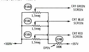
Symptom—Excessive brightness with retrace lines Cure—Check R248, and replace if it is open
