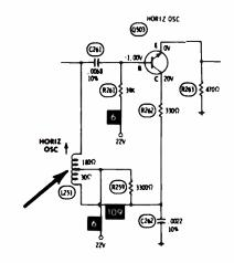
The defect was a loose core in the horizontal-oscillator coil. Apparently, it would vibrate from any mechanical movement and cause a shift of frequency.
