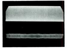
(B) Locking the scope to audio frequencies can be all that's necessary. Top trace is the oscillator signal (unmodulated) which is so far out of lock that it appears like a rectangle without detail. Even so, the height indicates the amplitude. Lower trace is a modulated carrier found at the loop antenna. It's there only when a station is tuned in, while the oscillator signal is there always.
