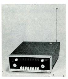
A typical eight-channel base/mobile scanner receiver.
