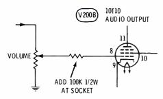
Symptom—Burned volume control because of tube arcs Cure—After replacing the volume control and tube, install a 100K resistor in series with grid wiring at the socket
