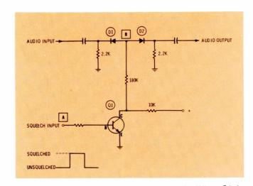
Fig. 8 Circuit of one type of audio squelch. When Q1 is cutoff, B+ flows through the 10K and 180K resistors to forward bias D1 and D2, and they pass the audio with very little distortion. When Q1 conducts there is no bias voltage on the diodes, and they become open circuits to squelch the audio.
