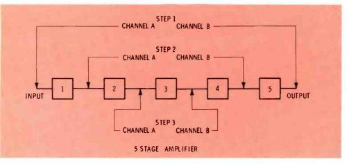
Fig. 12 Steps to zeroing-in on the origin of an intermittent.
