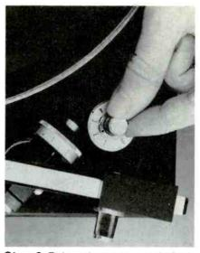
**Step 9** This alternate anti-skate system incorporates springs underneath the baseboard. They apply sideways pressure to the tone arm to counter any skating tendency. Ordinary adjustment calls for anti-skate pressure equal to stylus pressure. When done right, the anti-skate adjustment "balances" the tone arm in the lateral plane.
