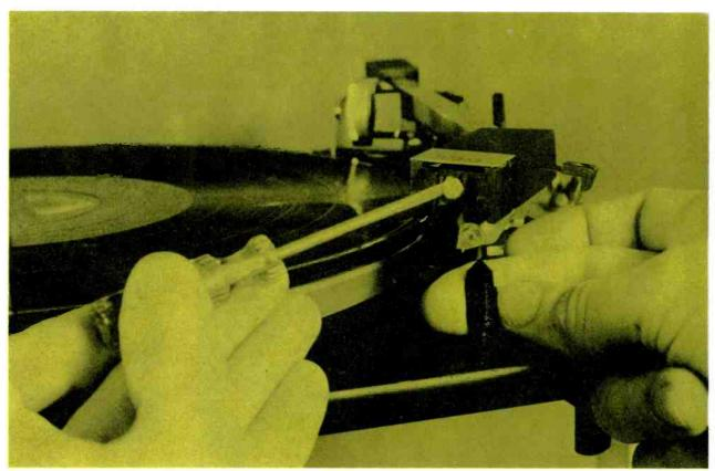
**Step 11** The lateral tracking adjustment puts the tone arm at the stylus on precisely the right tangent to the circle formed by the record grooves. This introduces the least possible tracking distortion. On the machine illustrated here, a guide post lets you determine where the exact tangent is; you align the stylus tip with the apex of the post.
