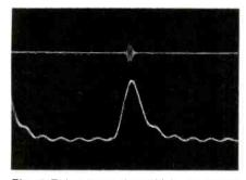
Fig. 5 False burst (spook) is produced at the plate by operation during a b-w program.
