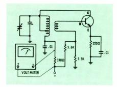
Fig. 1 In this oscillator circuit the collector current can be checked by measuring the voltage drop across the 330-ohm resistor, and then calculating the current by using Ohms Law. In the same way, check the emitter current by the voltage drop across the 220-ohm emitter resistor. Base voltage can be measured without adverse capacitive effects at the junction of the 5.6K and 3.3K bias resistors.
