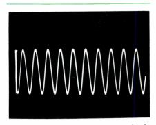
(A) A triggered-sweep scope locks easily to this AM oscillator of about 1.06 MHz. Amplitude can be measured by the scope calibrations.
