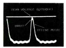
Fig. 6 Use the DC function with dual trace to measure the true bias voltage of the burst keyer tube at the tip of the keying pulse.
