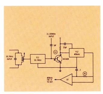
Fig. 7 Details of the dual 10.7-MHz/455-KHz IF circuit using ceramic crystal filters to give sharp selectivity.
