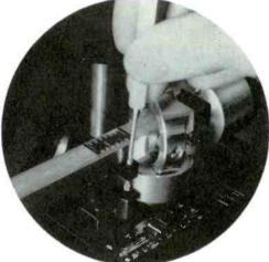
**Step 14** The tone arm, when it lifts during the change cycle, must raise high enough to clear records on the platter but not high enough to bump those stacked on the spindle. Above and to the left, respectively, are adjustments that control these limits.
