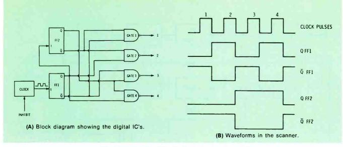
Fig. 4 Circuit and waveforms of a four-channel scanner.
