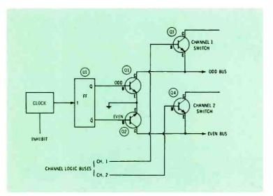
Fig. 5 Odd/even selection logic allows two four-crystal circuits to scan eight channels.
