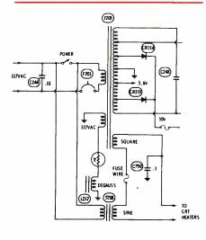
voltage regulation and a nearsquare waveform. Also, notice from the schematic that the heater should have below-normal sinewave power applied during the "off" time, and sufficient square waves during the "on" time. Because of the waveforms, we must consider the ability of different meters to give true or false readings. In this case, we measured the p-p amplitude of the heater voltage and found it to be too low.
