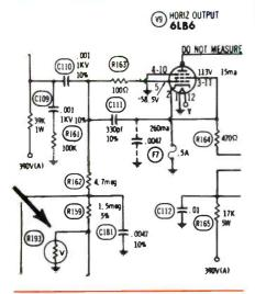
Measurement of parts in the high-voltage regulator circuit showed the varistor (R193) to be open. Probably it was arcing internally in the circuit.
