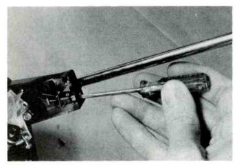
**Step 1** To adjust pressure that tone arm of record changer puts on stylus, you alter spring tension at vertical pivot. Inexpensive models have only rough adjustment—you shift the spring anchor point.
