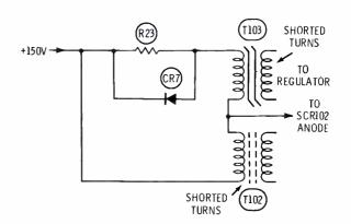
Symptom—Breaker opens following SCR replacements Cure—Check for shorted turns in T102 and T103
