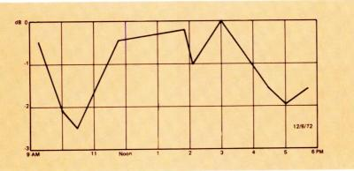
Fig. 3 Fringe signal-strength measured in one test lasting nine hours. During the time necessary to change antennas, the signal strength might change significantly.
