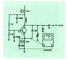
Fig. 2 Minimize any capacitive loading in this emitter circuit. It's better to measure the voltage drop across R1, in the collector circuit.
