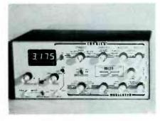
Model 1700A generates six carrier waveforms including sine, triangle, square, ramp, sawtooth, and pulse. The carrier frequency range is from 1 Hz to 1.5 MHz in twelve overlapping ranges. Included are three internal AM or FM modulator waveforms: sine, triangle, and square. The frequency range of the modulator wave-
