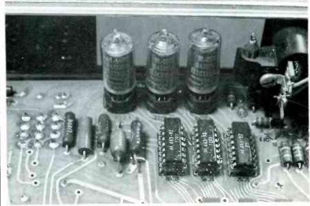
This partial view inside a Heathkit IM-102 shows the Nixie tubes and a few of the IC's.
