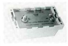
High-input capability of 228,000 dBmV reduces overload in areas having both weak and strong signals, and the 75-ohm coax minimizes noise pickup. The high output level provides enough signal in most areas to operate several TV sets.
