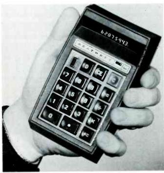
Typical of the four-function calculators is the Heathkit IC-2009 (Courtesy of Heath)
