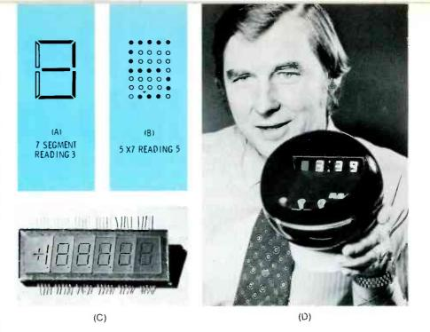
Fig. 6 Displays are segmented so all numbers from zero to nine can be formed by lighting the proper segments. (A) A 7-segment display looks this way when showing number 3. (B) A 5X7 35-segment display forms number 5. (C) A 5-1/2 digit gas-discharge display. (Courtesy of Diacon, Inc.) (D) An experimental electronic clock using liquid-crystal readout. (Courtesy of RCA)
