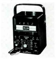
The new digital VOM features 29 AC, DC, and resistance ranges including low-power ohms. An analog output jack on the front panel makes it easy to interface with recorders and other instruments. Maximum fullscale response time to within rated accuracy is 2 seconds on DC, 5 seconds on AC. The unit operates from rechargeable batteries or AC line and may be operated while it is being charged.
