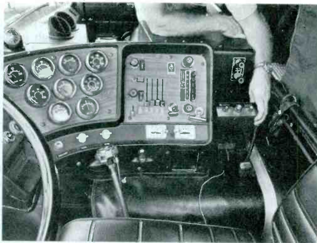
Fig. 1. In many trucks, a CB radio might interfere with movements of the driver's leg, if mounted under the dash in the usual way (left). Sometimes sufficient room can be found around the center console of a cab-over-engine model (right). Be sure the space isn't needed for something else, and that the driver can reach the CB controls and hear the speaker.
