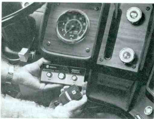
Fig. 1. In many trucks, a CB radio might interfere with movements of the driver's leg, if mounted under the dash in the usual way (left). Sometimes sufficient room can be found around the center console of a cab-over-engine model (right). Be sure the space isn't needed for something else, and that the driver can reach the CB controls and hear the speaker.
