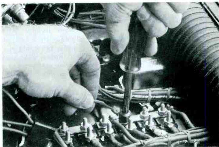
Fig. 7 With your test meter, find a DC-voltage bus that permits the driver to operate the CB rig even when power to the truck is off. Securely tighten the nut that holds the lug.
