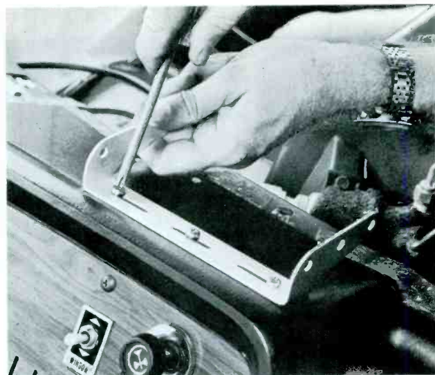
Fig. 5 If you're lucky and observant, you might find screws already located where they can hold the radio mounting bracket solidly.
