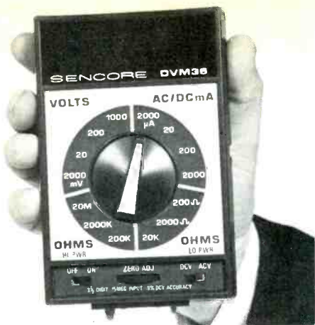
Fig. 4 Although the DVM36 appears to be nearly identical to the DVM35, it has 3-1/2 digits, permitting overranging up to 1999 instead of stopping at 999, and has a basic accuracy of 0.5% for DC voltages.
