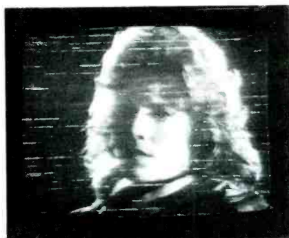
Fig. 8 Noise that isn't synchronous with either the vertical or the power line appears at random, without any pattern. This noise was made by a brush-type motor.
