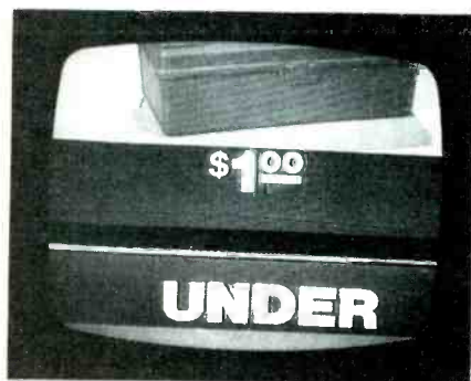
Fig. 1 When the picture and blanking bar move slowly down the TV screen, is the vertical sweep too slow so the video moves ahead of it on the way to the bottom of the screen? Or is the sweep too fast and moves part way to the bottom before the blanking bar arrives?
