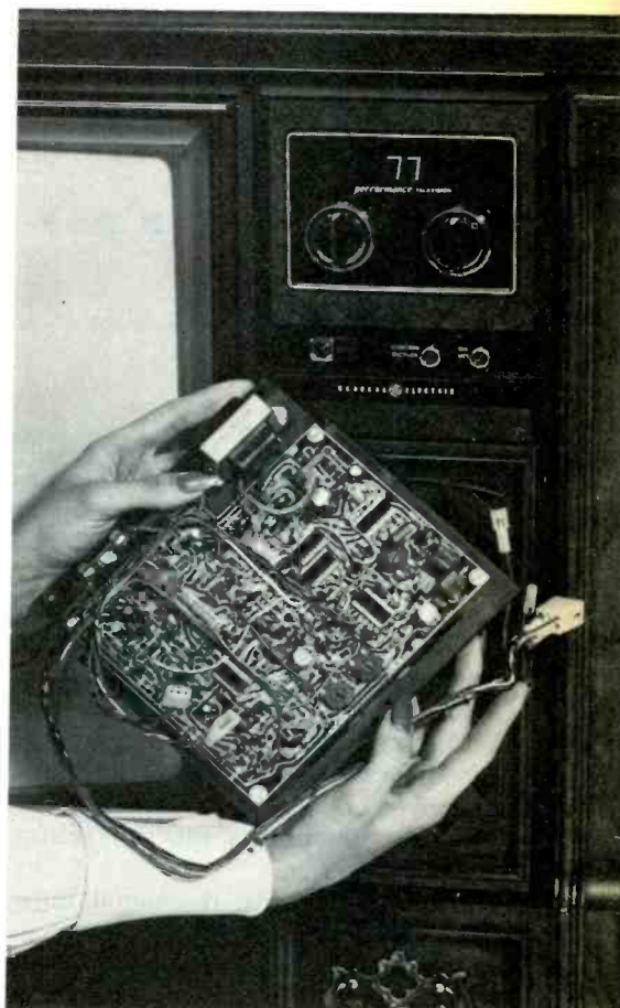
Fig. 2 Size of the module containing the GE VIR "Broadcast-Controlled" color circuitry is contrasted with one of the new receivers using it. Digital readout of switching-type tuners is another feature.
