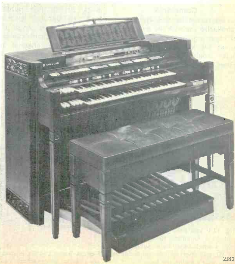
Fig. 11 The new Hammond Concorde organ is similar in appearance to the older models with tone wheels, but the circuits are all-solid-state with IC's and transistors. DC through the keyboard switches controls the sine waves.
