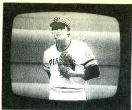
Fig. 6 These shaded areas have been called "silicon-diode radiation", but that's wrong. Instead, they are modulation bars caused by a change of signal strength from conduction of the power-supply diodes. They can't be seen unless there is a carrier which can be modulated.
