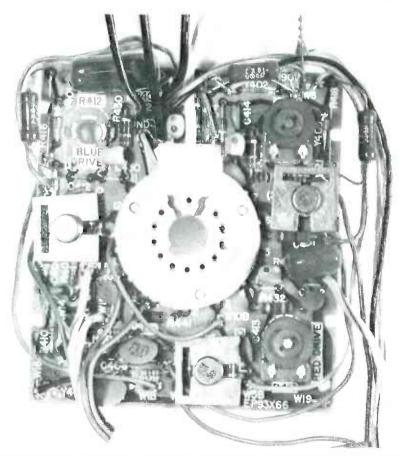
Fig. 8 Front side photo of the EP93X66 combination CRT-socket and matrixing module shows the three power transistors with their heat sinks.
