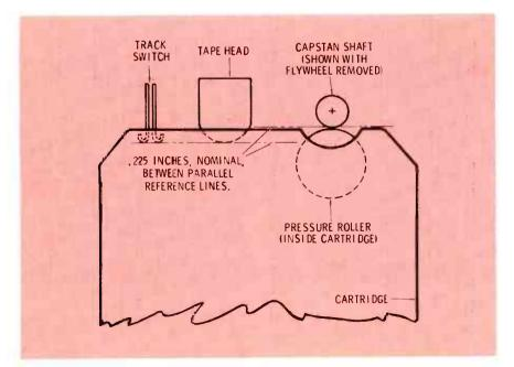
Fig. 12 The head should extend into the cartridge by approximately 0.225 inch. Notice that the track switch and the head are in line.
