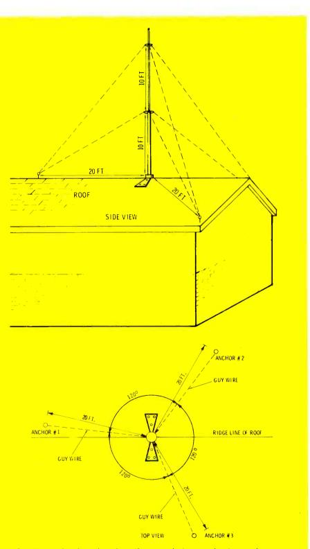
Fig. 8 These sketches show how the guy wires are to be arranged.
