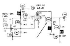
Back at the bench, I found less than -30 volts at the control grid of the horizontal-output tube. After wasting some time checking the components of the biasing network, I finally used the scope to find the grid drive was only about a third of the usual 300 VPP.
