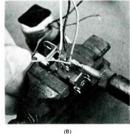
**Fig. 4** Before making new connections, match up the color codes with the diagram. Then, if the colors don't match, mark down the colors you assigned to the new cable. Keep as many as possible of the original colors (A). Check against the diagram as you solder the wires (B).
