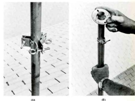
Fig. 7 Two kinds of collars or hubs commonly are used to anchor the guy wires to the mast. One (A) clamps to the mast with eye bolts, with the wires fastened through the eyes; and the other (B) is a collar with holes (thimbles should be used to minimize wear of the wires) for the guy wires. A pipe clamp is fastened underneath the collar to hold it into place
