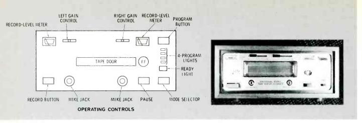
Fig. 1 The Zenith Model F638 is a deluxe tape deck (no power amplifiers) that both plays and records in stereo using 8-track cartridges. Meters show the recording level, lights indicate which of the four stereo programs is operating, and a "fast-forward" button switches in another motor winding that gives a faster tape speed. AC bias reduces the noise level and distortion during recording.
