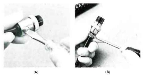
**Fig. 6** After the connectors are soldered and assembled, take these precautions to prevent shorts or an early failure. (A) Tighten the connector screws snugly, but don't use so much force that the threads are stripped or the insulator body is broken. (B) Don't squeeze the strain-relief so tight that it bites through or smashes the insulation.
