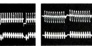
**Fig. 4** Waveform at the top is the 1-VPP color-bar pattern at the input to R210, before the take-off coil. Below is the 0.1-VPP color-bar "comb" pattern at the input of IC210 at pin 5.
