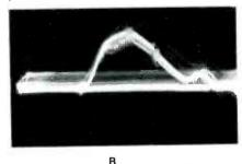
Fig. 11 Horizontal-sweep pulses are the "grass" that widens these alignment curves. The lower amplitude of the solid-state curves makes the pulses appear stronger. It was not convenient to kill the horizontal sweep because it also is the AC source for several DC power supplies. Curve (A) is the overall picture-IF response from tuner to the video; a type of "haystack". At (B), the curve shows the overall response from the tuner to pin 4 of IC270, using video-sweep modulation.
