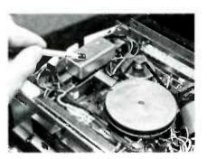
Fig. 20 The bias module has no adjustments and it is sealed. Replace it, if you suspect it has a defect.
