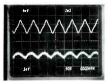
Fig. 19 One defective head gave this normal output (above) and the noisy, distorted one (below) from the other channel. It's good technique to check one channel against the other.
