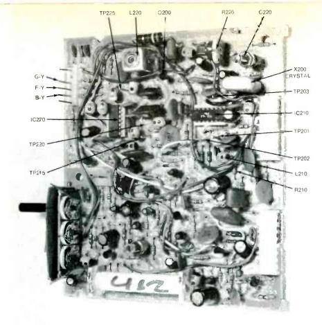
Fig. 1 Chroma circuits of the General Electric YC-2 chassis occupy less than half of the EP93X108 module.
