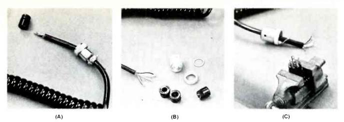
Fig. 5 Mike connectors are manufactured in many different variations. (A) This one comes with the screw-adjustable strain relief assembled ready to be slipped over the cable before the wires are soldered. Another kind (B) must be assembled as you go. (C) After the parts are installed on the cable, the wires are soldered to the connectors. Soldering is quicker and less-susceptible to wiring errors if you hold the connector block in a vise or vise-grip pliers.
