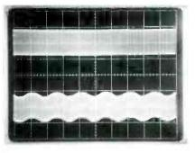
Fig. 21 Waveforms at the head during recording can give you much information. The correct waveform is below, with low-frequency sine waves and larger amplitude bias frequencies. Audio alone, without bias, would indicate a defect in the bias module. Bias without any audio (top trace) indicates a defect in the audio stages.
