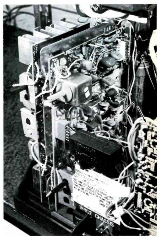
Both the video and chroma circuits are on the EP93X108 module, except for the final color power amplifiers on the CRT-socket module.
