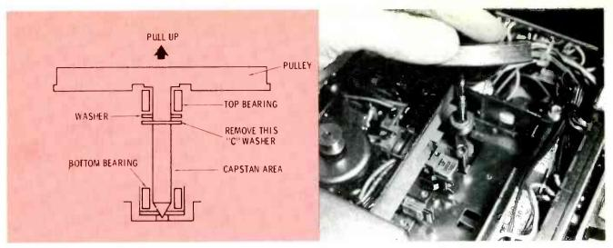
Fig. 9 The flywheel/pulley assembly must be removed to reach the head. First, remove the "C" washer (drawing) and the belt, then lift up on the assembly, as shown in photo.
