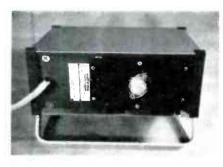
**Fig. 4** A large heat sink on the rear of the 244 easily dissipates the heat from the 2.5 amperes that CB radios require during transmissions.
