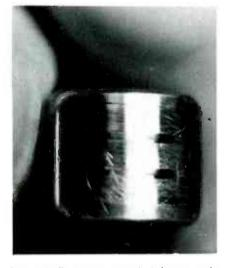
Fig. 18 Of all the head defects, only gap wear, and a scratched or dirty face shows in a visual inspection.
