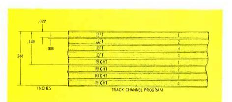
Fig. 7 Eight tracks, which are used as four stereo pairs, are recorded on the  $\frac{1}{4}$ " tape. Track 1 and 5 are the left and right stereo tracks of Program 1, tracks 2 and 6 are for Program 2, etc.
