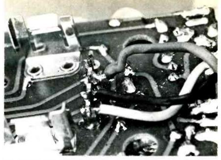
**Fig. 1** A hidden break of a wire at the terminal block inside a microphone does not require a new cable. Merely unsolder the open wire, clip it just behind the break, re-strip, and re-solder to the terminal.
