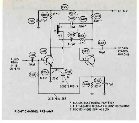
**Fig.** 3 Amplification and frequency compensation are functions of the 2-transistor pre-amplifier section. C403 bypasses the emitter of Q401, boosting the treble by reducing the emitter degeneration at high frequencies. In addition, the bass is boosted during playback by the values of C405 and R407 (A). DC stabilization of the direct-coupled stages operates by taking the base DC voltage for Q401 from the emitter of Q402. Each channel has a pre-amplifier.
