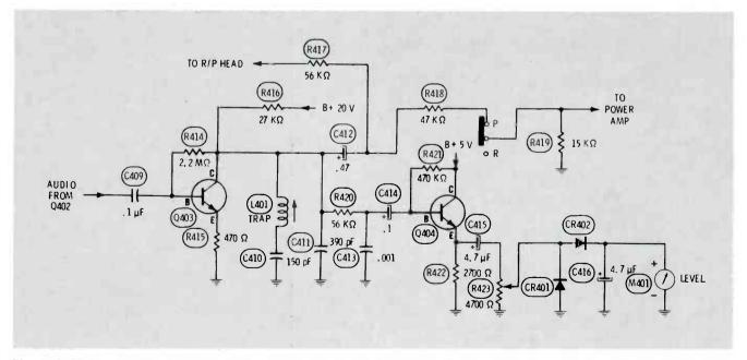
Fig. 4 Q403 is a simple amplifier with a tuned trap (L401 and C410) at the collector to remove any bias frequencies coming back from the head through R417. Output of Q403 goes to the head for recording (through R417), to the external power amplifiers (through R418), and to the emitter follower, Q404, which drives the meter rectifier and the recording meter. A similar circuit is provided for the other stereo channel.
