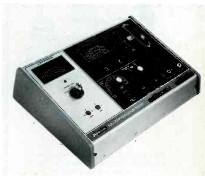
Figure 1 Model 530 semiconductor tester from B&K-Precision checks solid-state devices in three separate ways. Operation is rapid and positive, without ambiguous readings.
