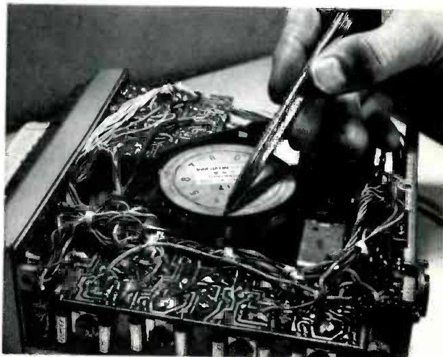
Figure 10 (Top) Remove the flywheel and capstan shaft assembly before you clean out the old grease and apply fresh lubrication to the bearing shaft.
