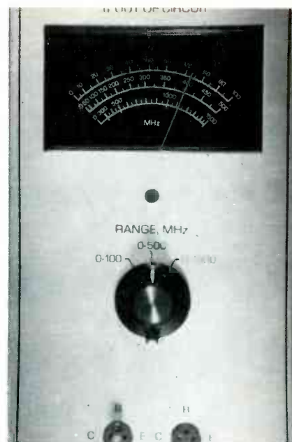
Figure 4 Controls, meter, and circuitry for measuring the frequency where a bipolar transistor gives a gain of one are at the left. They are completely separate from the controls for the other tests. A test frequency of 1 MHz is used for the 100-MHz range; 10 MHz for the 500-MHz range; and 30 MHz for the 1500-MHz range.
