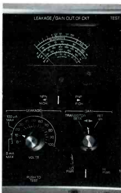
Figure 3 In the center of the panel are found the controls and meter for out-of-circuit leakage and gain measurements.
