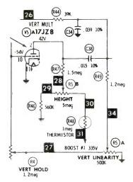
After I had replaced a filter capacitor and a resistor, the set was placed on time test. After a time I noticed tearing of the picture horizontally near the top of the picture.
