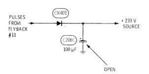
$\ensuremath{ \mbox{Symptom-No}}\xspace$  video, and excessive brightness with retrace lines
