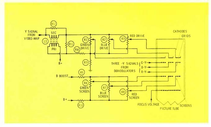
Figure 1 Almost all tube-equipped color receivers matrixed the video (Y) and chroma (-Y) signals inside the picture tube, as shown. The precise DC voltages at the control grids, screen grids, and cathodes affect the brightness or gray-scale screen color and tracking. An open in the
