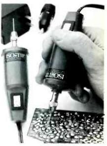
The drill's compact size allows use in confined areas and within cabinetry. High impact plastic housing makes it lightweight and an extra-long 10-ft. cord provides a wide working radius. On/off switch provides both "intermittent-on" and "locked-on" positions.
