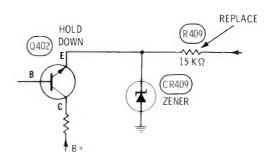
Symptom—Vertical lines at the edges are crooked Cure—Check R409, and replace it if out of tolerance
