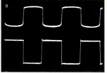
Figure 6 The top trace of photo A is the clipped output from D128, and the bottom trace is the output waveform from D129. Photo B shows the base waveform (top trace) and the collector waveform (bottom trace) of Q120, which acts as a 60-Hz clock.
