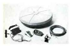
The unidirectional antenna of the Mini-State system can be rotated by a hand-held remote control unit. The UHF-VHF antenna rotates inside a weather-protected polyethelene radome, which also houses a solid-state amplifier, interference filter, and a motor-driven rotator.
