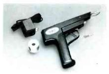
A plug-in battery charger comes as standard equipment, and it will fully recharge the nickel-cadmium batteries overnight. The tip comes up to full soldering heat within 5 to 10 seconds, and performance is said to equal a conventional soldering iron. A "lock-off" switch prevents accidental heating of the tip while the iron is in storage or during transportation.
