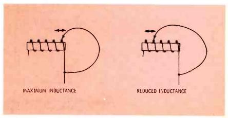
**Figure 4** A shorting bar or shorting jumper gives the effect of removing turns from a coil, thus decreasing the inductance.
