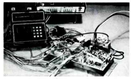
Most of the cables to the panel unit and the control chassis are long enough (after the cable ties are removed) to permit locating the panel and chassis on a table or bench near the TV. Only two extender cables are required, and they can be obtained from Magnavox. All components of the Touch-Tune system are easily accessible, and all functions can be operated, when the two units are removed from the cabinet.
