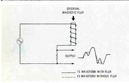
Figure 8 External magnetic fields can be detected by phase and linearity changes of the output signal. The external flux aids one peak of the input AC, but it subtracts from the opposite peak.
