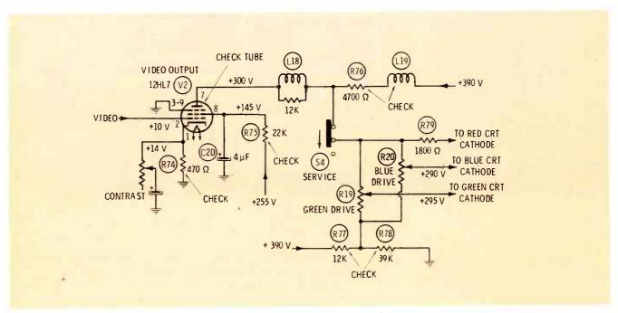
Figure 5 In a Zenith 16Z8C50, excessive gun currents had killed the high voltage. Use DC-voltage analysis to find similar problems.
