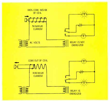
Figure 2 Position of an object can be sensed by connecting it to the core of a coil. (A) When the core is inside the coil, the coil inductance and inductive reactance are high, giving low current which does not trip the relay. (B) Withdrawing the core reduces the inductance, allowing increased current that trips the relay.
