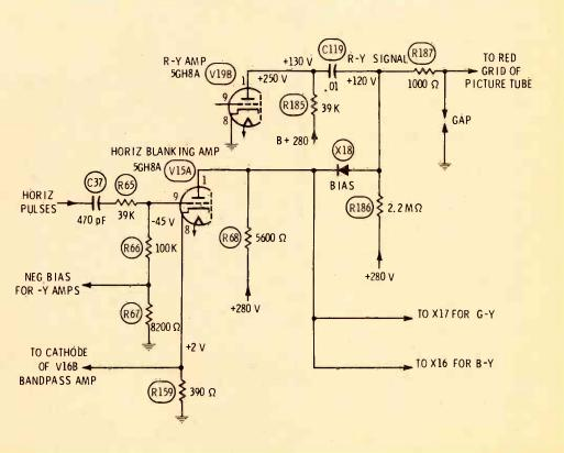
open diode or a leaky one drastically raises the DC voltage of the associated CRT grid. Therefore, the best test is to disconnect one end of any suspected diode and measure forward and reverse resistances by using an ohmmeter.
