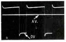
Figure 3 The bottoms of these waveforms are at zero DC volts. Therefore, each horizontal line represents the average DC voltage. The waveforms vary in pulse width (duty cycle), and thus produce different DC voltages after passing through three RC low-pass filters. The waveform on the left (A) was generated by channel 2, and the tuning voltage was +4.42; the wider pulses of the right waveform (B), channel 6, gave a tuning voltage of +21.2.
