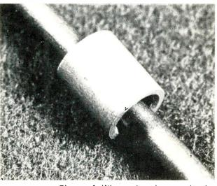
Figure 4 When placed around wire conductor, ferrite beads act as a small inductance. The advantage over coils is that the wire and bead do not have any self-resonance.
