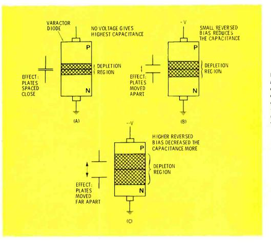
**Figure 2** Reverse bias applied to a junction diode changes the size of the depletion region, giving the effect of moving the plates of a capacitor to produce a varying capacitance.
