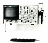
either a troubleshooting tool or a TV waveform monitor. The TV-sync separator provides improved locking at video horizontal and vertical rates. The scope can be powered from AC line, 12 VDC, or a selfcontained rechargeable battery with built-in charger.
