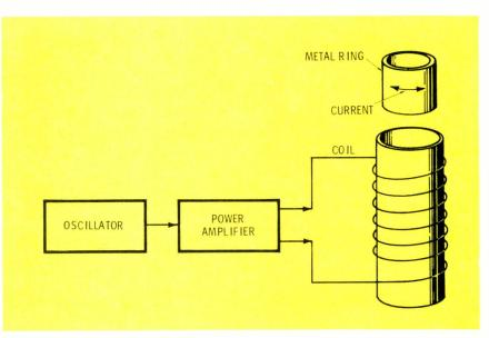
Figure 1 AC current in a metal ring placed in the field of an inductor produces heat. The RF frequency and the amount of power applied to the coil determines how hot the ring becomes. •
