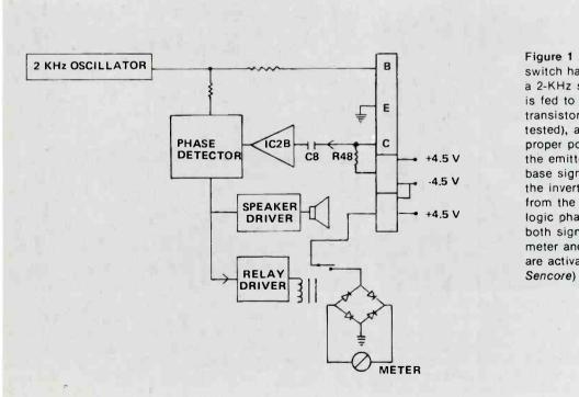
Figure 1 After the permutator switch has been set correctly, a 2-KHz square-wave signal is fed to the base of the transistor (that's being tested), and bias of the proper polarity is applied to the emitter. A sample of the base signal, and a sample of the inverted square waves from the collector, go to a logic phase detector. When both signals are present, the meter and the speaker tone are activated. (*Courtesy of* Sencore)
