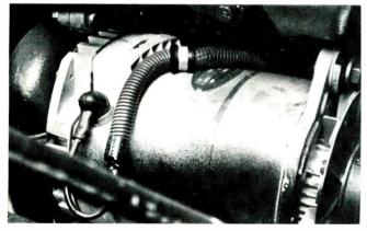
Figure 6 Newer alternators have built-in electronic regulation circuits, so no field wire or post is needed.
