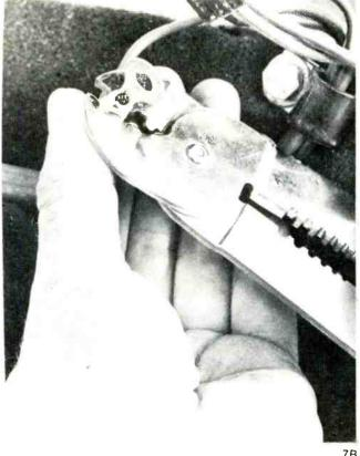
Figure 7 (A) Crimp lugs onto the ends of all wires (don't merely tin the lead and wrap it around a terminal). Strip  $\frac{1}{4}$ -inch of insulation, tin the strands, and insert into the
