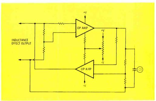
Figure 3 An inductance effect can be obtained by this circuit that uses opamps. The advantage over discrete coils is that such gyrator circuits can be made small enough to be included inside ICs.
