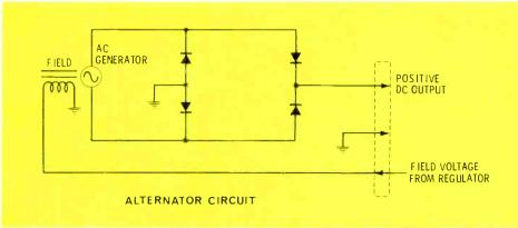
Figure 1 Alternators produce AC voltage, which is rectified by diodes. Noise sources include the slip-rings and brushes that feed power to the diodes, and the diodes themselves. Not all have the negative side grounded.
