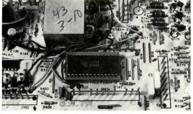
**IC103,** the control processor, is the largest one on the control chassis. It has 28 pins. Three of the ICs incorporate the new Integrated Injection Logic (called I squared L) that permits low-current drives; therefore, the "highs" are supplied at lower DC voltage levels than for other digital circuits.
