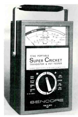
Model TF46 Portable Super Cricket Transistor And FET Tester from Sencore operates from internal battery cells. A door slides over the meter face, to protect it during transportation. The test lead compartment, at the bottom, is closed for the picture.
