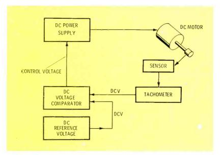
Figure 11 A speed control for a DC motor is similar to the one in Figure 10, except the reference and sensor signals are DC, the comparator works from those DC voltages, and the motor speed is changed by varying the applied DC voltage.
