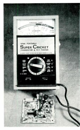
**Figure 4** The Sencore TF46 Super Cricket is shown giving a "good" Cricket in-circuit reading of a transistor on a Magnavox module.
