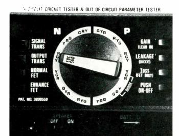
Figure 2 In the center is the permutator-switch pointer, which selects all combinations of leads and polarity. The eight pushbuttons at the sides select the conditions and functions. The gain, IDSS, and leakage buttons are the only ones that do not latch. The SPEAKER OFF/ON switch can be seen dimly at the left bottom; it is at the back of the storage compartment. The BATT TEST switch is shown at the right bottom corner.
