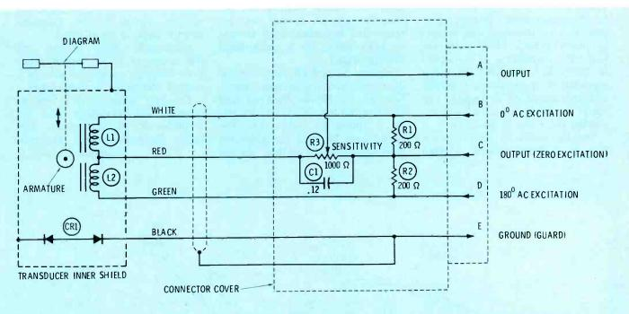
Figure 4 This is the internal circuit of Hewlett-Packard are mounted inside the large connector. Included is a 1280-series blood-pressure transducers. The three resistors graph of pressure versus output voltage.
