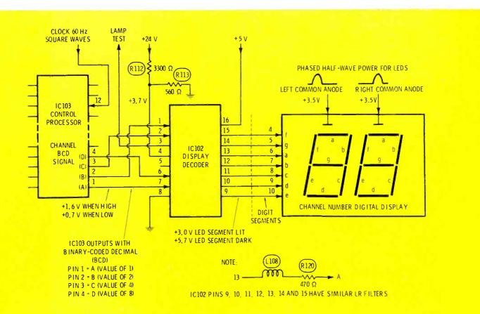
Figure 6 The display decoder, IC102, receives the A, B, C, and D lines of the BCD output from IC103 and changes the BCD to the logic required for lighting the seven-segment LED display. Multiplexing of the two channel digits is done
