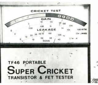
Figure 3 The five scales of the TF46 meter are, from top to bottom: good/bad Cricket and battery test; 0 to 500 beta for bipolar transistors; 0 to 25K microhms for FETs; 0 to 2,500 microamperes for transistor leakage; and 0 to 50 milliamperes for FET leakage.
