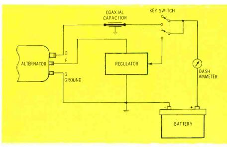
Figure 2 This block diagram of alternator wiring shows where the coaxial capacitor should be inserted, for best noise reduction. It should be mounted very near the DC-output post.
