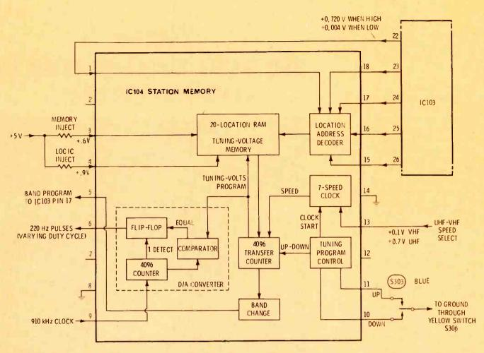
Figure 7 Internal functions of IC104 are shown by the blocks, with pin numbers in the proper sequence. The varying-width pulses of DC voltage from pin 6 are filtered
