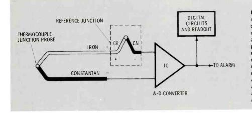
Figure 6 Accurate temperature measurements by a thermocouple device requires a reference junction, operated at the ambient temperature, that opposes the voltage from the measuring junction. The output can be increased by using multiple junctions. An analog meter can be used to read the output voltage, or (as shown) a digital circuit can activate an alarm and show the temperature on a decimal readout.
