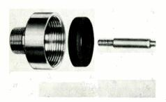
The model 41901, available as an accessory device, allows total interchangeability between Antenna Incorporated and Motorola antennas, or any other antennas using the Motorola-style mount. Designed to accommodate any standard baseloaded antenna, the mount fits over the Motorola mount with a special threading device, which then is attached to the female connection of the antenna.
