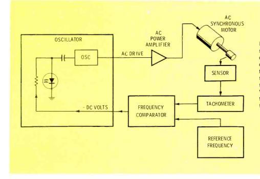
Figure 10 One type of speed control for a synchronous motor uses a closed-loop, and compares the tachometer reading of the motor speed against the reference frequency. Varying the frequency of the motor voltage changes the motor speed.
