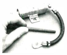
Figure 5 A round file or tapered reamer should be used to enlarge the mounting hole or terminal hole, as needed.
