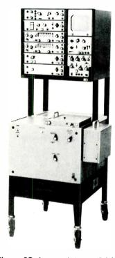
Figure 5C A complete model VR-6 physiological monitoring system by "Electronics For Medicine" includes two blood-pressure amplifiers with meters, plus a scope for viewing most of the waveforms from the various instruments. At the bottom is a strip-chart recorder, for permanent waveforms. (Courtesy of Electronics For Medicine)
