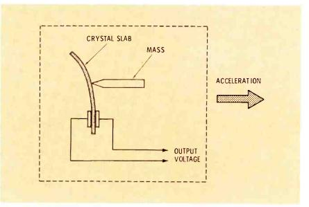
Figure 9 In an accelerometer, the signal from a crystal slab is in proportion to the amount of acceleration applied to the standard mass.
