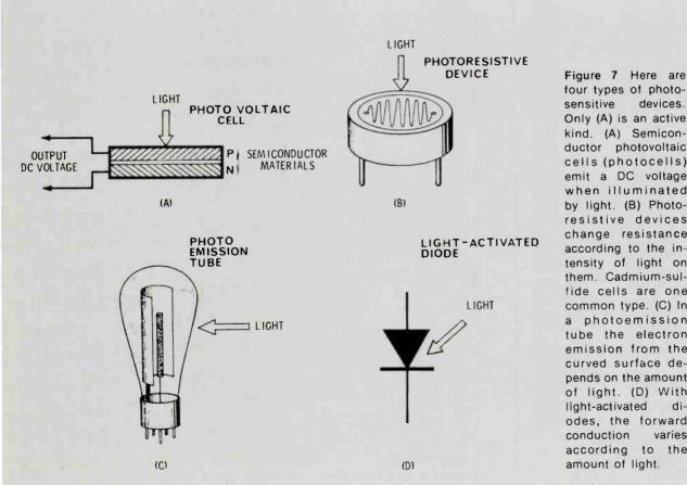
four types of photodevices. Only (A) is an active kind. (A) Semiconductor photovoltaic cells (photocells) emit a DC voltage when illuminated by light. (B) Photoresistive devices change resistance according to the intensity of light on them. Cadmium-sulfide cells are one common type. (C) In a photoemission tube the electron emission from the curved surface depends on the amount of light. (D) With light-activated diodes, the forward conduction varies according to the amount of light.
