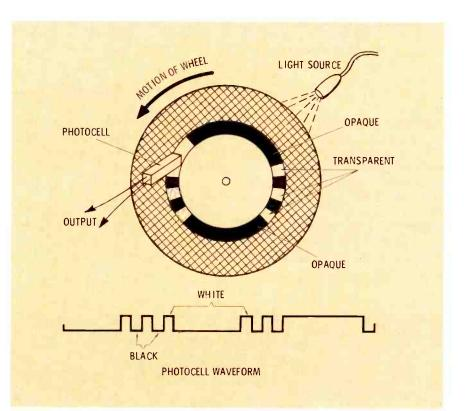
Figure 8 A rotating disc with transparent sections between a light source and the photocell can act as a digital encoder.
