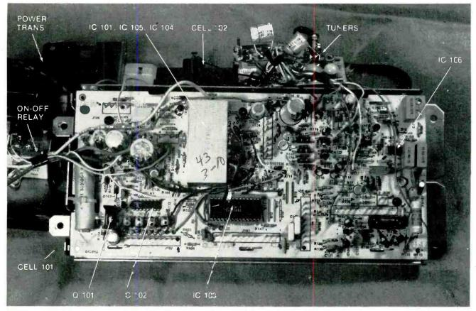
Figure 1 Major components of the Touch-Tune control chassis are indicated by the arrows.
